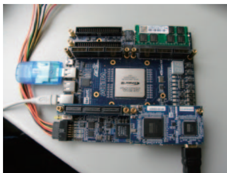
Fig. 14. FPGA board (DE3 board) used for the implementation.
