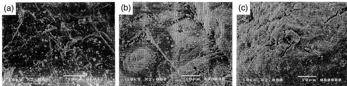
Fig. 1. SEM photographs of \text{CaCO}_3 calcined at 800^\circ\text{C} . (a) as received, (b) 1h and (c) 3h calcined.
