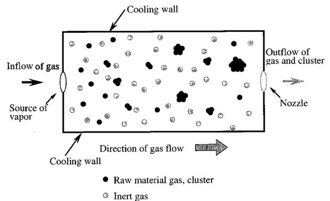
FIG. 1. Schematic illustration of the cluster growth apparatus. The large arrow indicates the rarefied gas flow of the raw material and inert gas. During the flow of raw material along the flight path cluster growth occurs.
