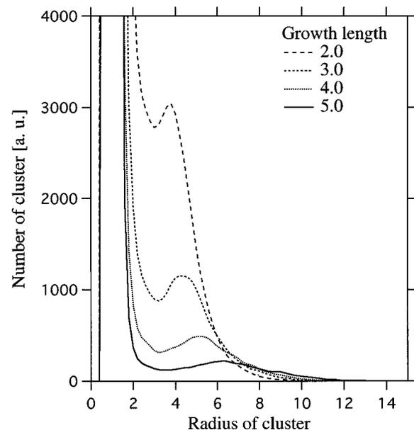
FIG. 2. Typical size distributions of the clusters at the nozzle. The concentration of the inert gas is 10% and the temperature of the wall is 1.0. The cluster radius is normalized by that of the monomer.
