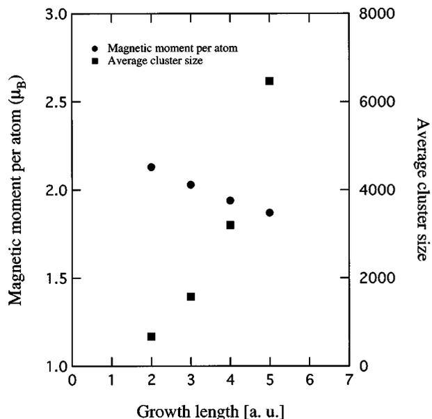
FIG. 3. Average magnetic moment per atom and average cluster size under various conditions corresponding to Fig. 2 as a function of the growth length.
