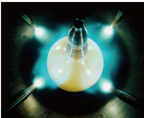
Fig. 1 Picture of single crystal growth using a tetra-arc furnace installed at IMR.
