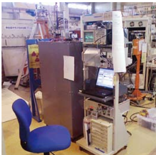
Fig. 1 A portable capacitor bank of neutron diffraction, which is installed at JRR3 reactor. It can be set into a limited space of a spectrometer.
