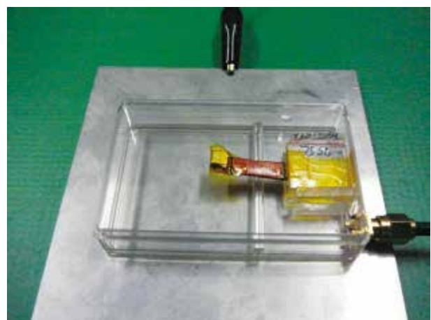
Fig. 2 Vibration-energy-harvesting device incorporating an Fe-Co alloy thin film.
