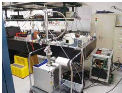
Fig. 2 Experimental Setup installed at Rice University, Houston. The box in the right is the capacitor bank, and the cylinder in the center is the cryostat with a magnet.
