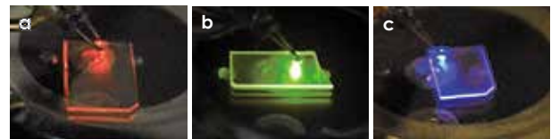
Fig. 2 Full-color RGB emission from In x Ga 1-x N/ GaN MQW LEDs with different indium contents x of (a) 0.40, (b) 0.29, and (c) 0.17.
