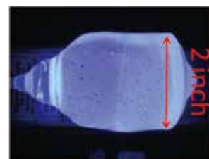
Fig. 2 2-inch La-GPS single crystal (as grown)
