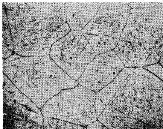
Photo. 9 Mn 42.9%, 750°×3 days, water quenched and 450°×52 hrs. tempered, etched by \text{NH}_4\text{OH}+\text{H}_2\text{O}_2 and \text{FeCl}_3+\text{HCl} , ×200.
