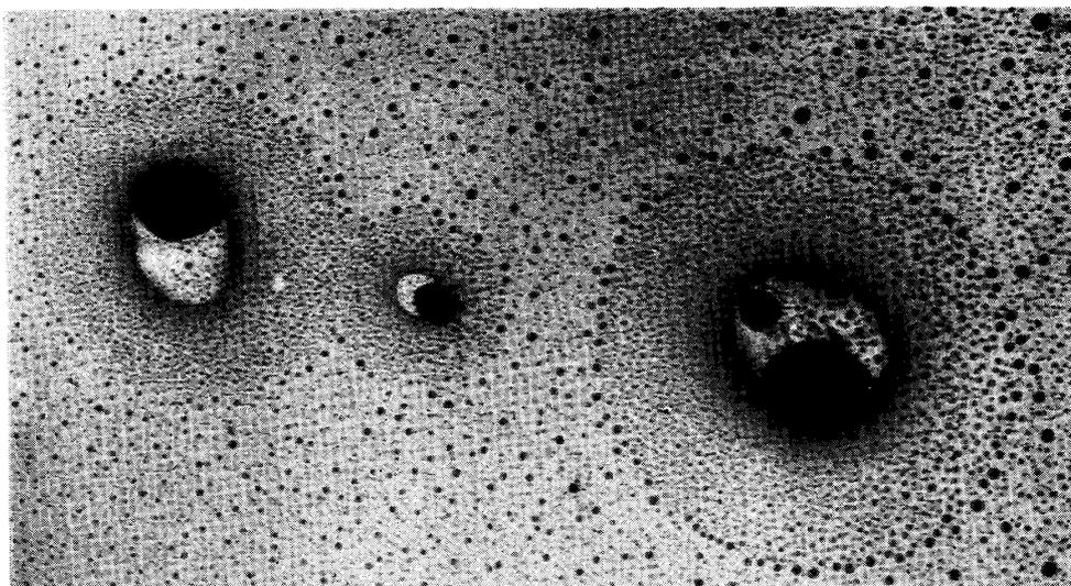
Fig. 9. Electron micrographs showing the unknown contamination deposited from the circumference of specimen supporter on the specimen already having the "halos" due to the electron bombardment. 28,000 $\times$
