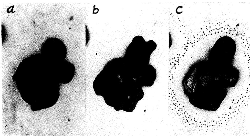
Fig. 2. Electron micrographs of the "Fuji" process emulsions in the case of medium thickness of gelatine before sensitization produced in the dark room. (a), (b) and (c) correspond to the cases of weak, intense and more intense electron bombardment, respectively.
