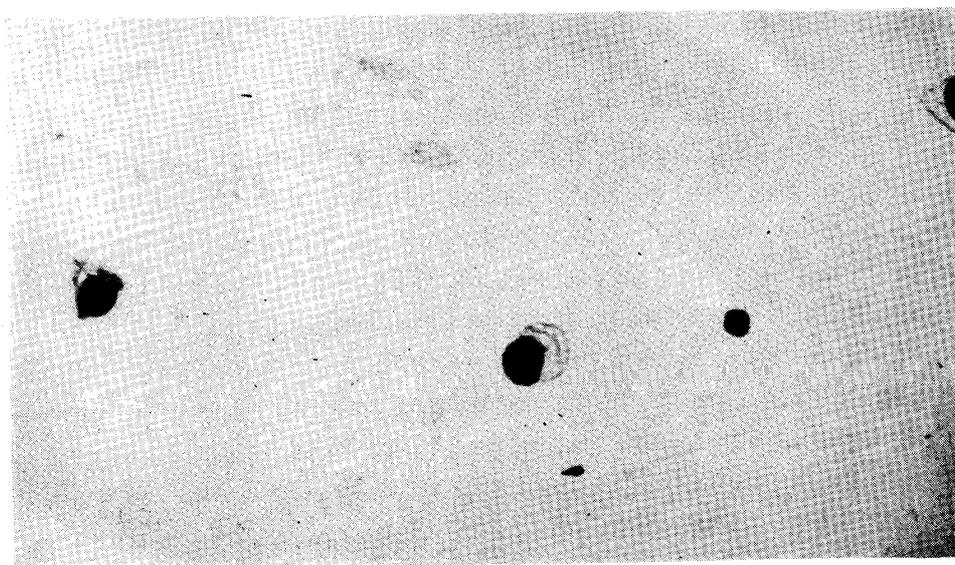
Fig. 7. Electron micrographs of the emulsions produced by the ripening of colloidal silver bromide without gelatine. 28,000 $\times$
