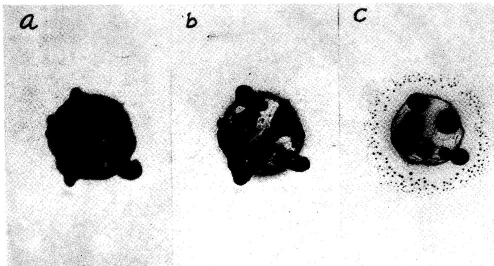
Fig. 1. Electron micrographs of the "Fuji" process emulsions in the case of medium thickness of gelatine after sensitization. (a), (b) and (c) correspond to the cases of weak, intense and more intense electron bombardment, respectively.
