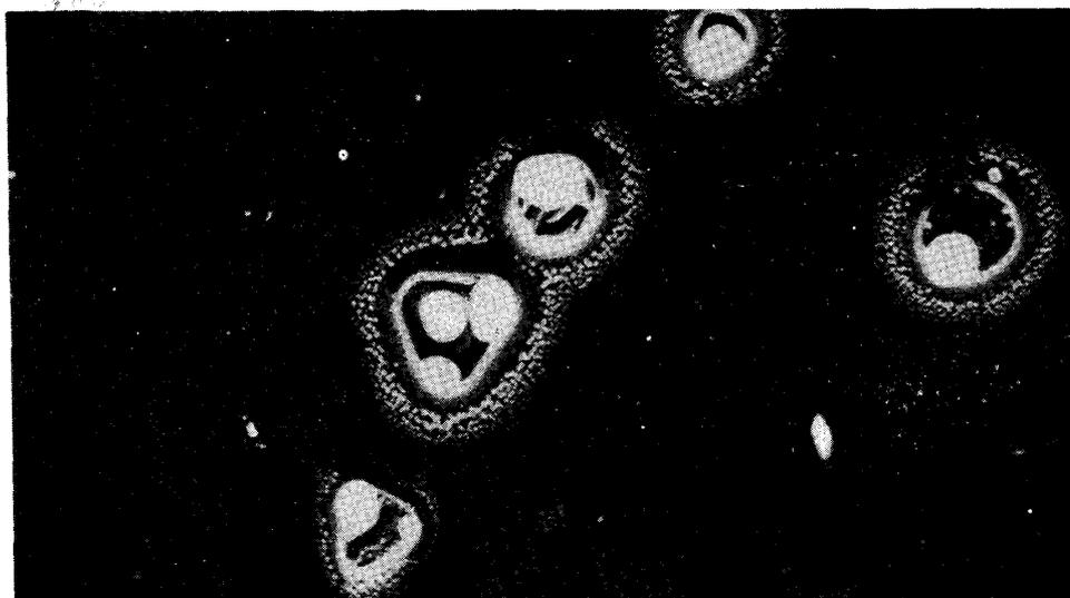
Fig. 8. Cr-shadowed electron micrographs of the "Fuji" process emulsions in the case of medium thickness of gelatine before sensitization. 22,000×
