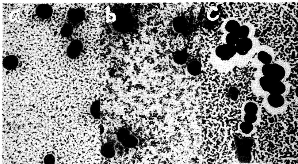
Fig. 10. Electron micrographs of the specimens of carbon black only, of carbon black placed on gelatine film, and of carbon black filled in gelatine film on the collodion foil, having very slightly deposited silver films under the same conditions ((a), (b) and (c)). 25,000 ×
