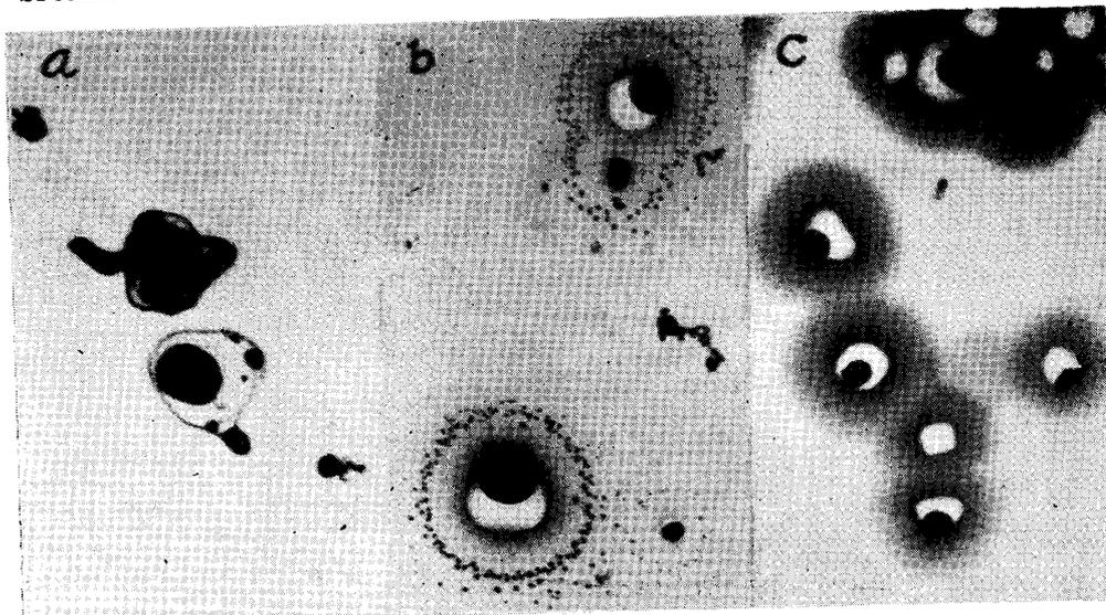
Fig. 6. Electron micrographs of the emulsions produced by the ripening of colloidal silver bromide in the cases of thin, medium and thick gelatine, respectively ((a), (b) and (c)). 28,000 $\times$
