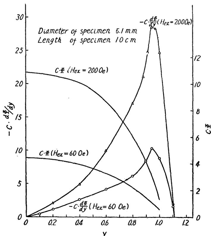
Fig. 2. The relations of magnetic flux  $\Phi$  and flux leakage  $-d\Phi/dy$  to the distance  $y$  from the center of the magnetized bar.
