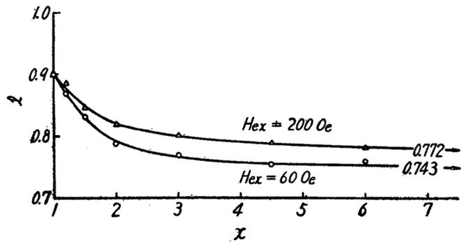
Fig. 3. The relations of the equivalent pole distance  $l$  to the distance  $x$  between the magnetometer and the center of the magnetized bar when the two coils are on the same axis.
