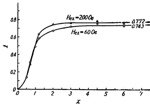
Fig. 4. The relations of the equivalent pole distance  $l$  to the distance  $x$  between the magnetometer and the center of the magnetized bar when the two coils are in parallel.
