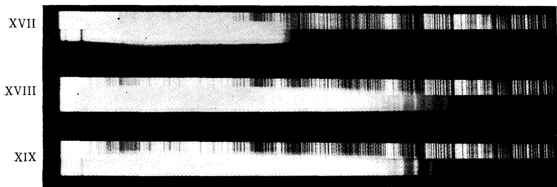
Condensed discharge with induction coil. XVII : liquid oxygen, XVIII : liquid nitrogen, XIX : liquid air.
