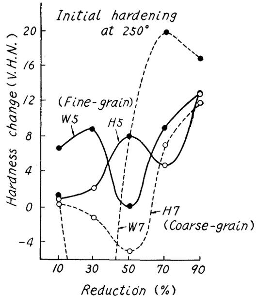
Fig. 4. Initial hardening at 250° of cold-rolled 70/30 brass sheets.
