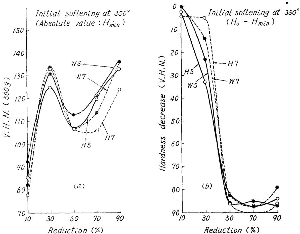
Fig. 6. Initial softening at 350° of cold-rolled 70/30 brass.
