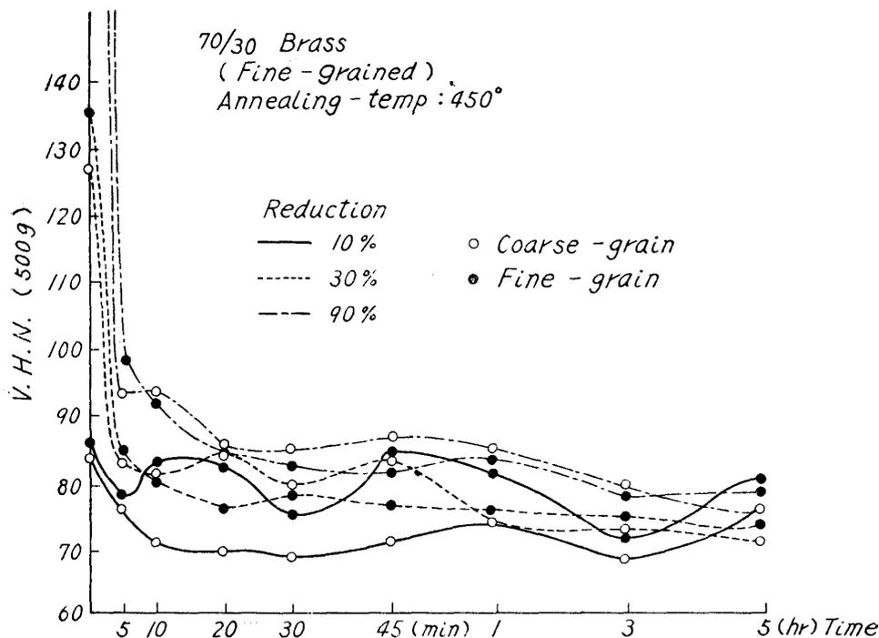
Fig. 8. Change in hardness at 450° of cold-rolled 70/30 brass.
