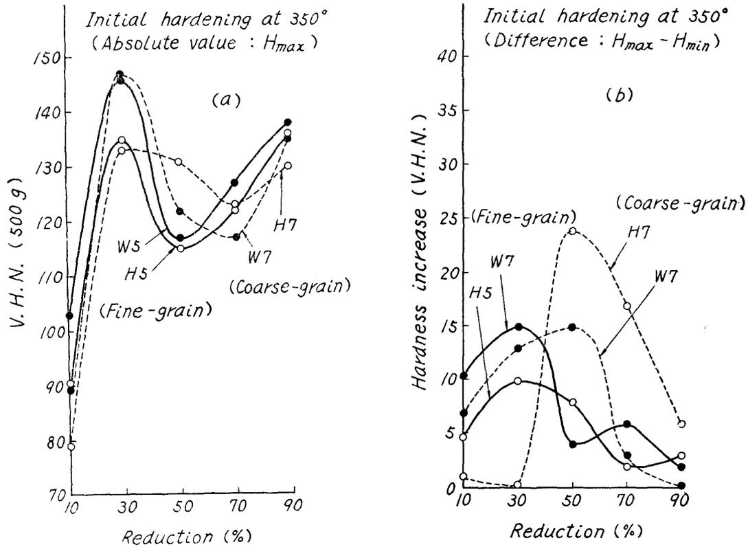
Fig. 7. Initial hardening at 350° of cold-rolled 70/30 brass.
