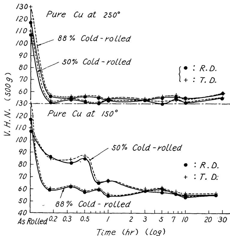
Fig. 9. Change in hardness at 150° and 250° of cold-rolled pure copper.
