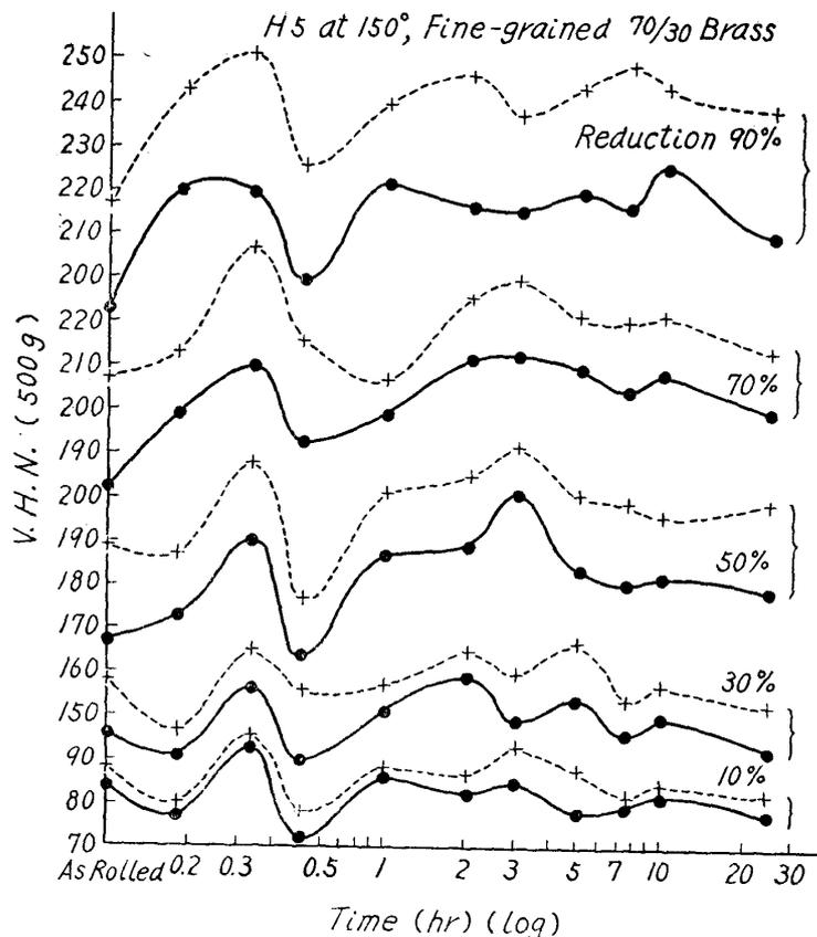
Fig. 1. Change in hardness at 150° of fine-grained, cold-rolled 70/30 brass, ● : Parallel to rolling direction, + : Transverse to rolling direction.
