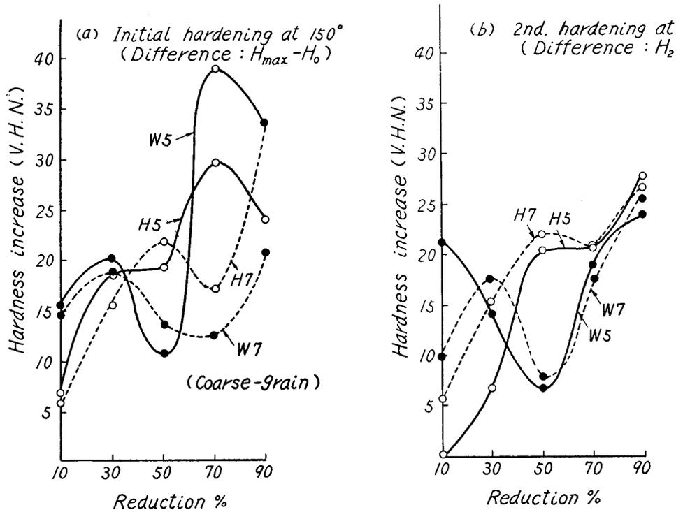
Fig. 2. Primary and secondary hardening at 150° of cold-rolled 70/30 brass sheets.
