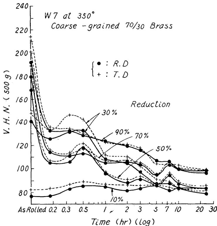
Fig. 5. Change in hardness at 350° of coarse-grained, cold-rolled 70/30 brass.
