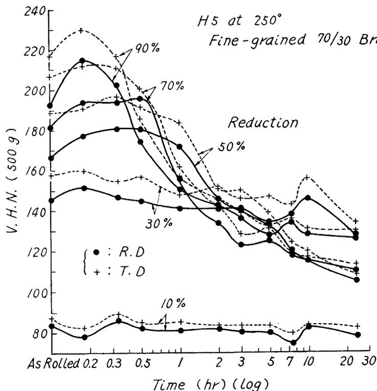
Fig. 3. Change in hardness at 250° of fine-grained, cold-rolled 70/30 brass.
