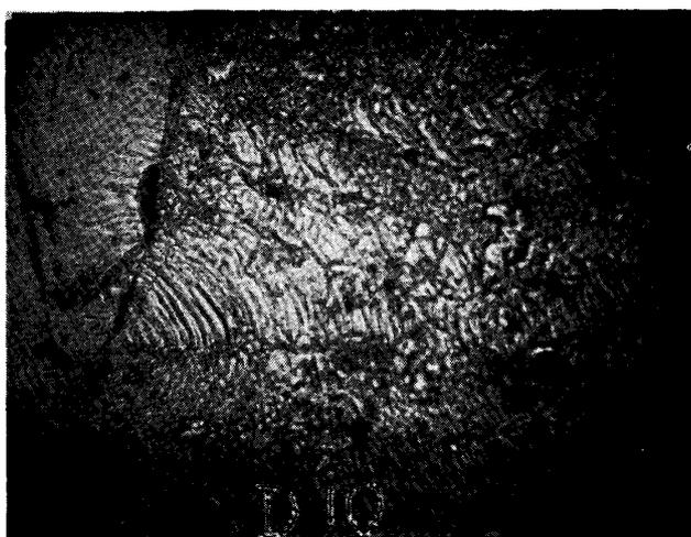
Photo. 13. Recrystallization in strain-marking region of cold-rolled 70/30 brass plate, reduction : 70%, annealed at 250° for 5 hrs, magnification :  $\times 1,046$
