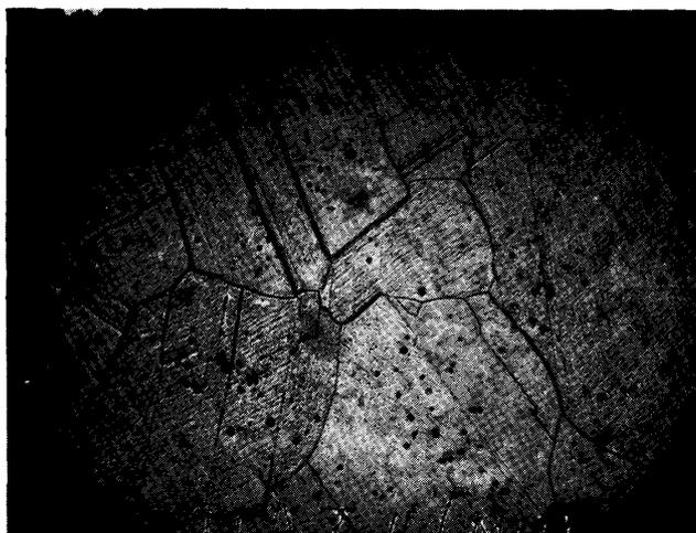
Photo. 1. Microstructure of plate surface of cold-rolled 70/30 brass, specimen : coarse-grained, reduction : 10%, magnification :  $\times 100$
