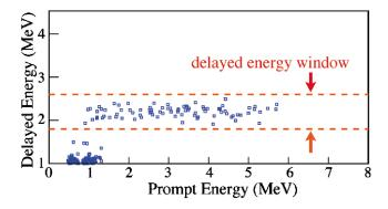
FIG. 3 (color). Distribution of  $\bar{\nu}_e$  candidates after fiducial volume, time, vertex correlation, and spallation cuts are applied. For  $\bar{\nu}_e$  events the prompt energy is attributed to positrons and the delayed energy to neutron capture. Events within the horizontal lines bracketing the delayed energy of 2.2 MeV are consistent with thermal neutron capture on protons.
