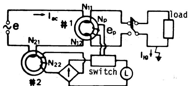
Fig. 7. Basic circuit of leakage current alarm device.
