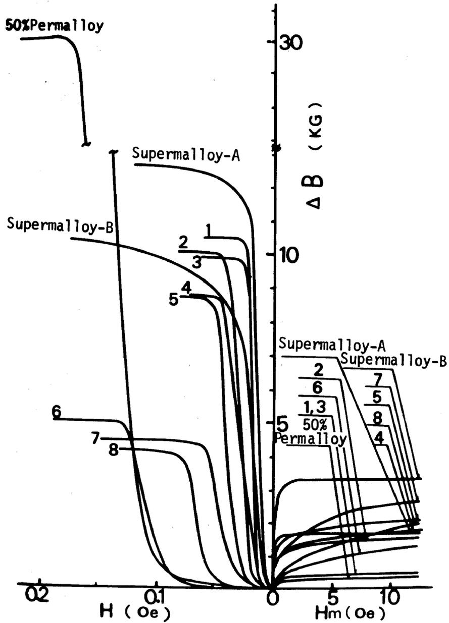
Fig. 2. Control magnetization curves indicated with magnetizing force  $H$  and flux density value  $\Delta B$ .
