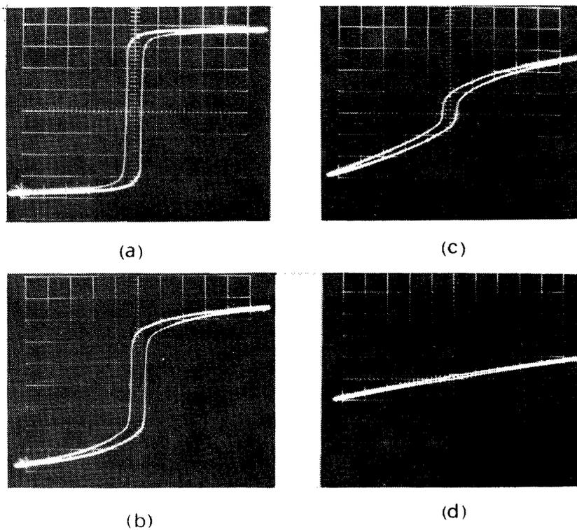
Fig. 5. Measured B-H loops of an amorphous core supplied with magnetizing force rotated  $90^\circ$ .
