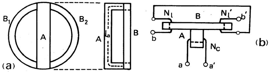
Fig. 9. Bridge-connected magnetic circuit using amorphous core. (a) Magnetic circuit. (b) Connection of windings.
