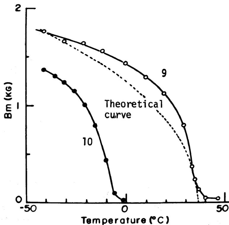
Fig. 6. Temperature sensitive magnetic characteristics of amorphous cores.
