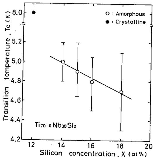
Fig. 12 Silicon concentration dependence of the superconducting transition temperature ( $T_C$ ) and the transition width ( $\Delta T_C$ ) for  $\text{Ti}_{70-x}\text{Nb}_{30}\text{Si}_x$  amorphous alloys. Vertical bars represent the transition width.
