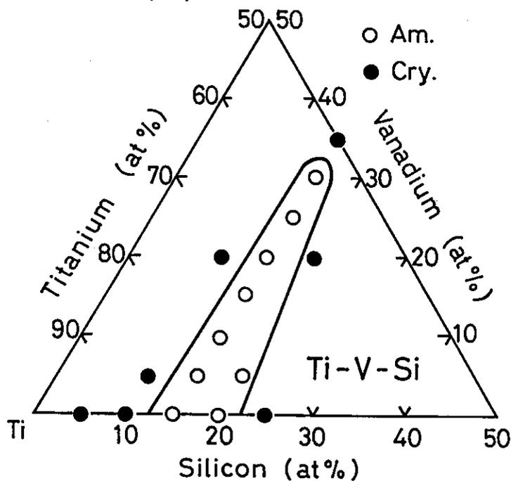
Fig. 5 Composition range for formation of amorphous phase in Ti-V-Si ternary system.
