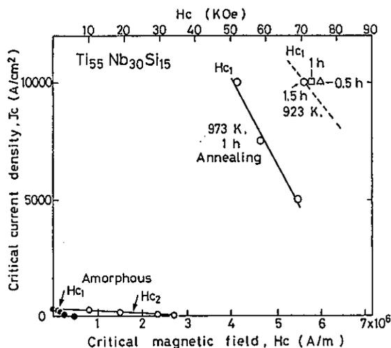
Fig. 34 Critical current density ( $J_C$ ) of  $Ti_{55}Nb_{30}Si_{15}$  amorphous alloy annealed for 0.5 and 1 h at 923 and 973 K as a function of magnetic field applied normal to the direction of current flow.
