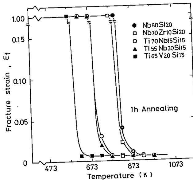
Fig. 7 Change in fracture strain by annealing for 1 h at various temperatures for  $\text{Nb}_{80}\text{Si}_{20}$ ,  $\text{Nb}_{70}\text{Zr}_{10}\text{Si}_{20}$ ,  $\text{Ti}_{85-x}\text{Nb}_x\text{Si}_{15}$  and  $\text{Ti}_{65}\text{V}_{20}\text{Si}_{15}$  amorphous alloys.
