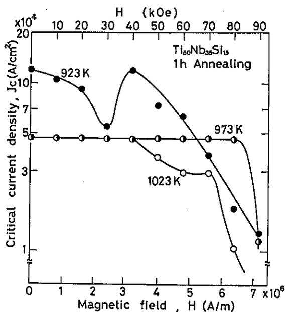
Fig. 35 Critical current density ( $J_c$ ) of  $Ti_{50}Nb_{35}Si_{15}$  amorphous alloy annealed for 1 h at various temperatures as a function of magnetic field applied normal to the direction of current flow.
