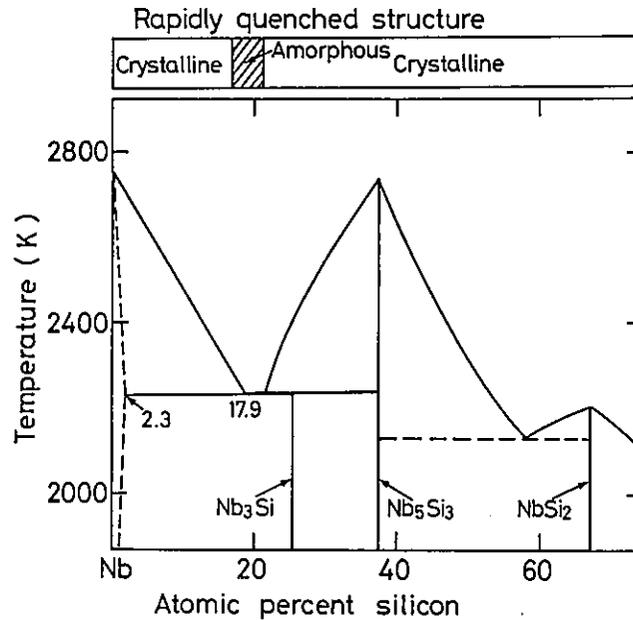
Fig. 2 Composition range for formation of amorphous phase in Nb-Si binary system. Binary phase diagram was obtained from Ref. [17].
