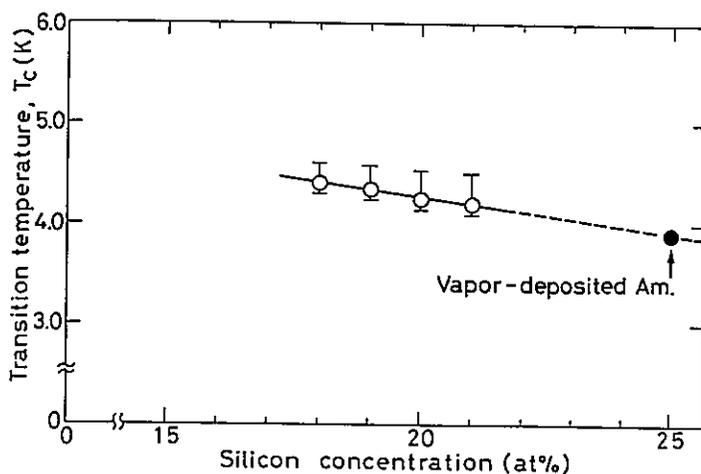
Fig. 8 Silicon concentration dependence of the superconducting transition temperature ( $T_C$ ) and the transition width ( $\Delta T_C$ ) for Nb-Si amorphous alloys. Vertical bars represent the transition width.
