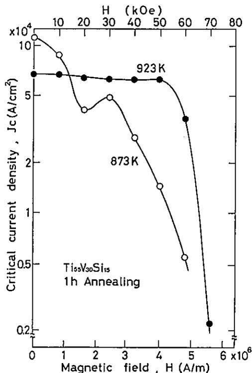
Fig. 37 Critical current density ( $J_c$ ) of  $Ti_{55}V_{30}Si_{15}$  amorphous alloy annealed for 1 h at 873 and 923 K as a function of magnetic field applied normal to the direction of current flow.
