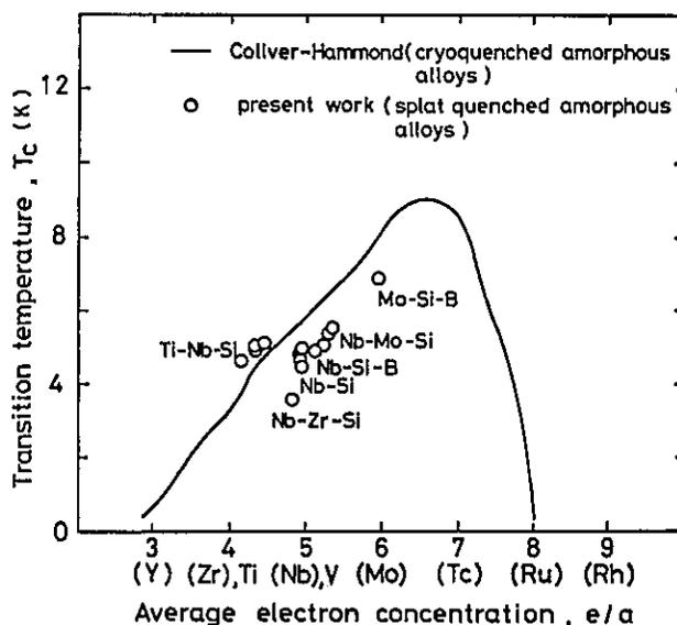
Fig. 13 Superconducting transition temperature( $T_C$ ) versus electron per atom ratio for the 4d transition-metals series. The data for the amorphous vapor-quenched films were taken from Ref. [26].
