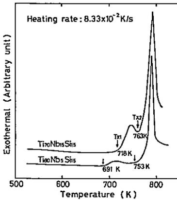
Fig. 25 Differential thermal analysis curves of  $Ti_{80}Nb_5Si_{15}$  and  $Ti_{70}Nb_{15}Si_{15}$  amorphous alloys.
