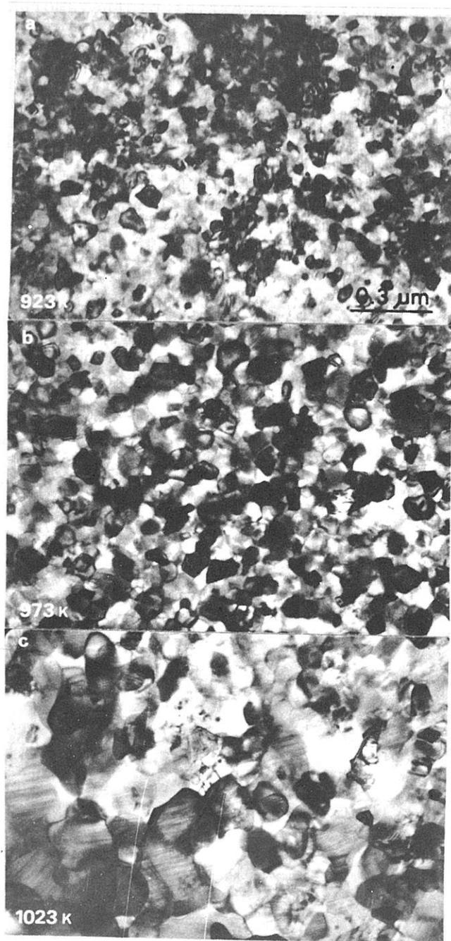
Fig. 38 Transmission electron micrographs of  $\text{Ti}_{50}\text{Nb}_{35}\text{Si}_{15}$  amorphous alloy annealed for 1 h at 923 K(a), 973 K(b) and 1023 K(c).
