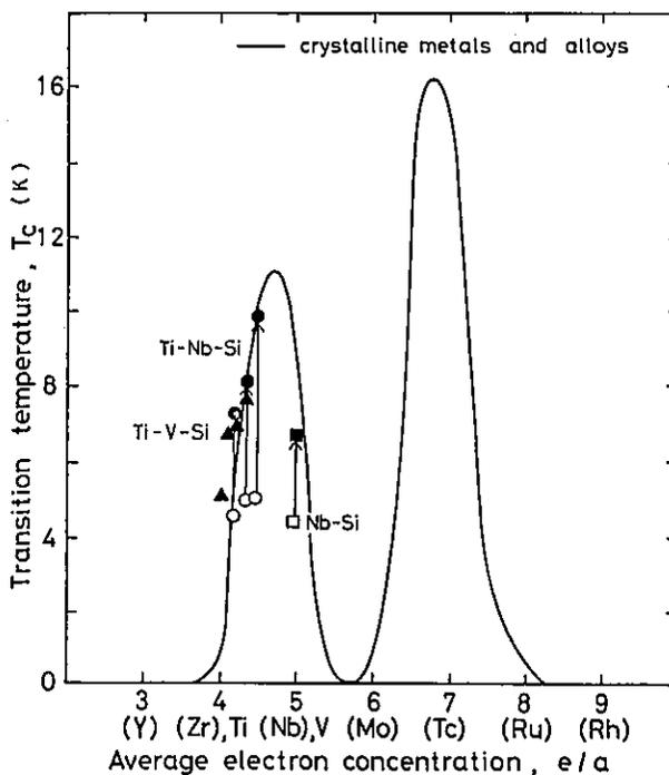
Fig. 32 Superconducting transition temperature ( $T_C$ ) vs. electron per atom ratio ( $e/a$ ) for the 4d transition-metal series.
