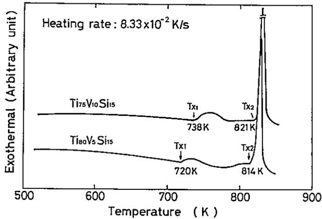
Fig. 26 Differential thermal analysis curves of  $Ti_{80}V_5Si_{15}$  and  $Ti_{75}V_{10}Si_{15}$  amorphous alloys.
