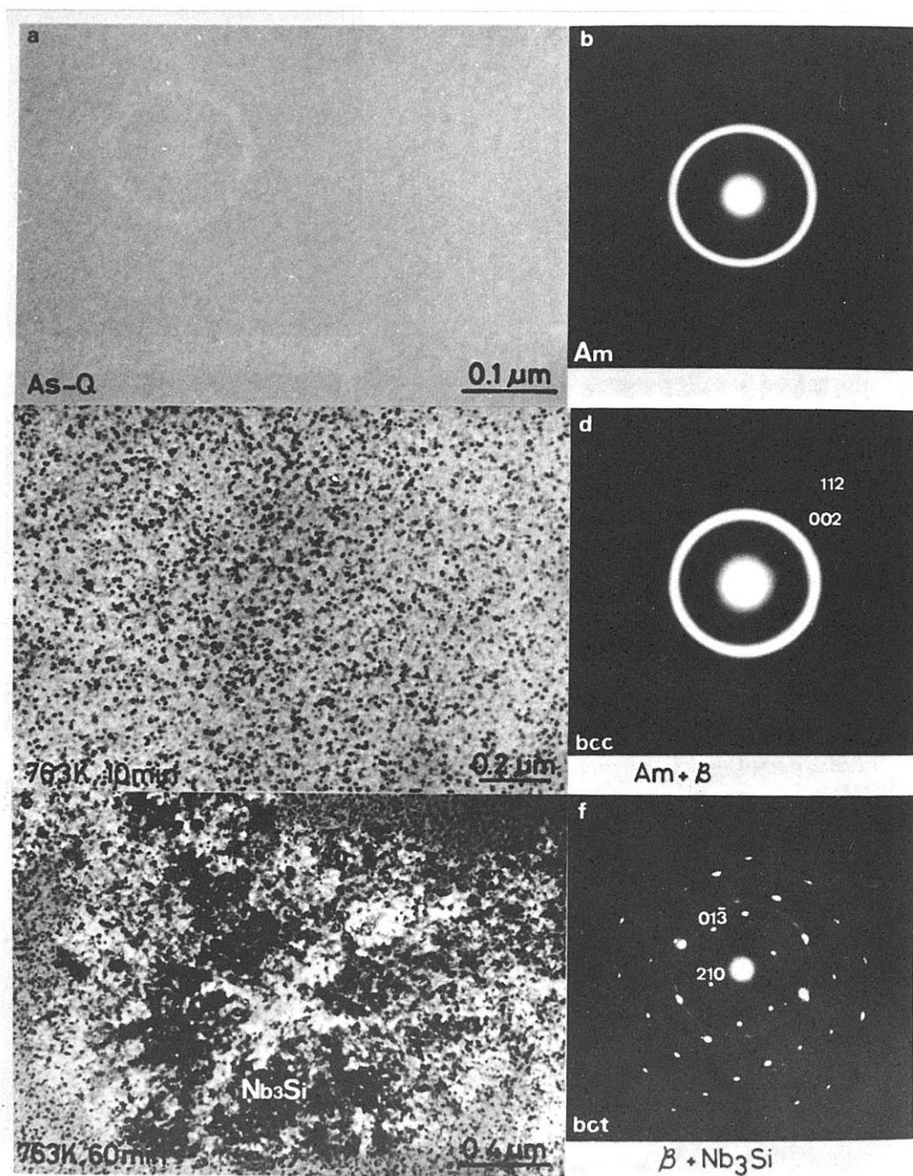
Fig. 27 Transmission electron micrographs and selected area diffraction patterns showing the as-quenched (a and b) and annealed (c, d, e and f) structure of  $\text{Ti}_{70}\text{Nb}_{15}\text{Si}_{15}$  amorphous alloy.
