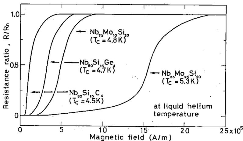
Fig. 17 Resistance ratio  $R/R_n$  as a function of magnetic field at liquid helium temperature for several Nb-based amorphous alloys.
