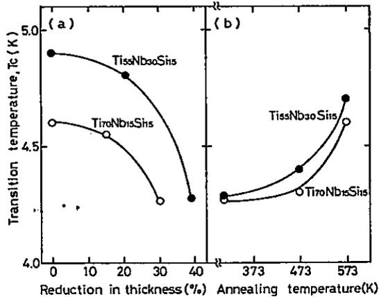
Fig. 14 (a) Change in superconducting transition temperature ( $T_c$ ) of  $Ti_{70}Nb_{15}Si_{15}$  and  $Ti_{55}Nb_{30}Si_{15}$  amorphous alloys by cold rolling. (b) Change in superconducting transition temperature ( $T_c$ ) of cold-rolled  $Ti_{70}Nb_{15}Si_{15}$  and  $Ti_{55}Nb_{30}Si_{15}$  amorphous alloys by annealing.
