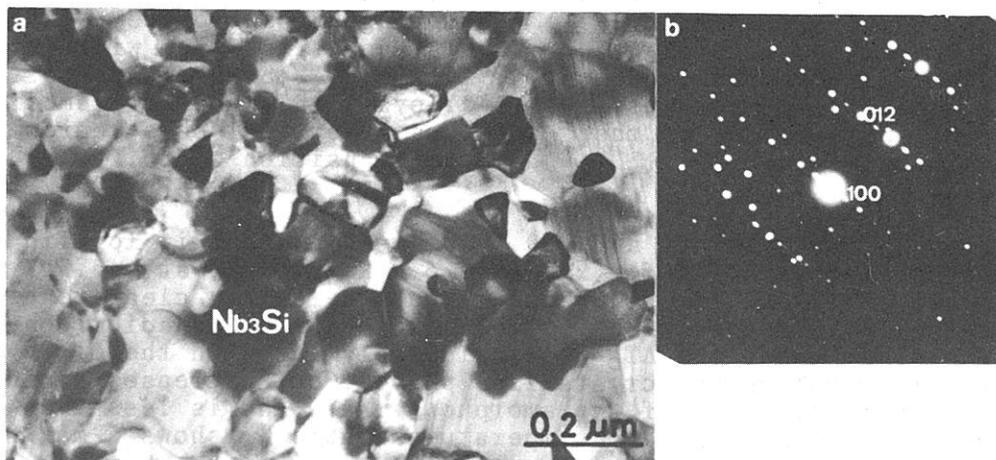
Fig. 29 Transmission electron micrograph and selected area diffraction pattern of Ti<sub>70</sub>Nb<sub>15</sub>Si<sub>15</sub> amorphous alloy annealed for 1 h at 833 K.
