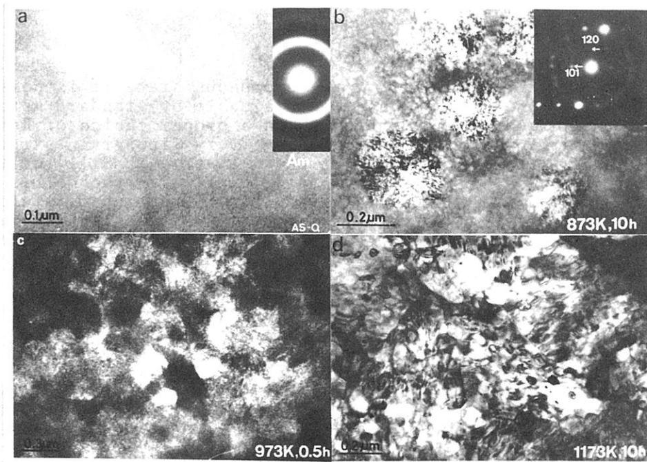
Fig. 22 Transmission electron micrographs and selected area diffraction patterns showing the microstructures of  $Nb_{80}Si_{20}$  amorphous alloy heated for different periods at various temperatures.
