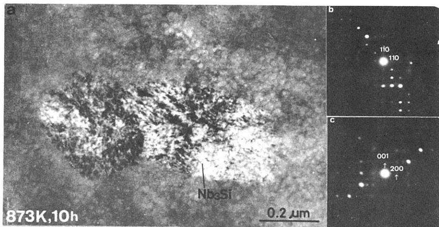
Fig. 23 The morphology and crystalline structures of  $Nb_3Si$  compound for  $Nb_{80}Si_{20}$  amorphous alloy heated for  $10h$  at  $873K$ . (a) bright field image, (b) and (c) selected area diffraction patterns taken from the crystals in the photograph (a). The normals to the crystals are  $[001]$  and  $[010]$ , respectively.
