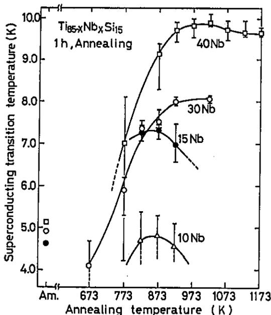
Fig. 30 Changes in superconducting transition temperature ( $T_C$ ) and transition width ( $\Delta T_C$ ) for  $Ti_{85-x}Nb_xSi_{15}$  amorphous alloys with annealing temperature. Vertical bars represent the transition width.
