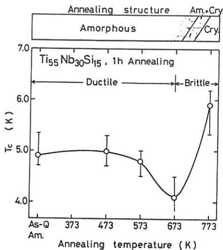
Fig. 15 Change in superconducting transition temperature ( $T_c$ ) of  $Ti_{55}Nb_{30}Si_{15}$  amorphous alloy upon annealing for 1 h at various temperatures.
