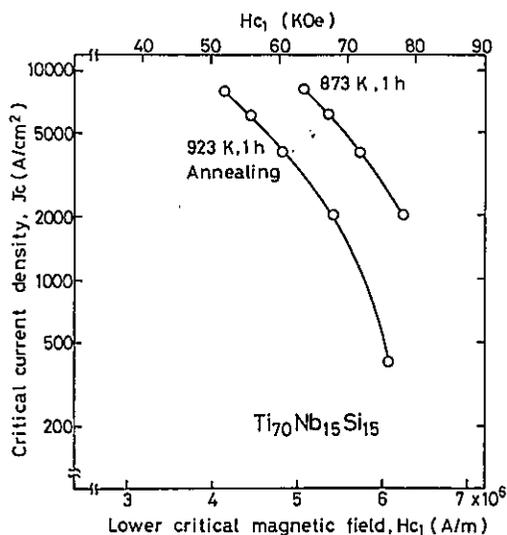
Fig. 33 Critical current density ( $J_C$ ) of  $Ti_{70}Nb_{15}Si_{15}$  amorphous alloy annealed for 1 h at 873 and 923 K as a function of magnetic field applied normal to the direction of current flow.
