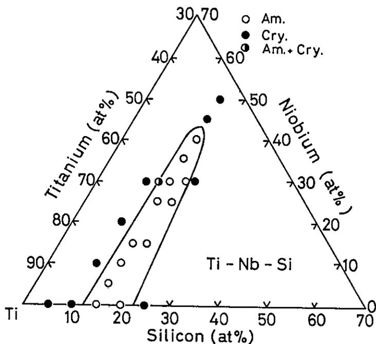
Fig. 4 Composition range for formation of amorphous phase in Ti-Nb-Si ternary system.
