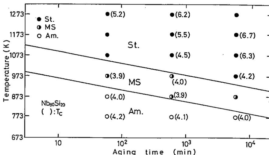
Fig. 24 The superconducting transition temperature ( $T_C$ ) of  $Nb_{80}Si_{20}$  amorphous alloy annealed for different periods at various temperatures.
