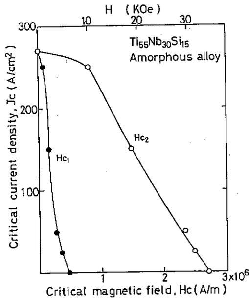
Fig. 20 Critical current density ( $J_c$ ) of  $\text{Ti}_{55}\text{Nb}_{30}\text{Si}_{15}$  amorphous alloy as a function of magnetic field applied normal to the direction of current flow.
