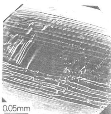
Fig. 6 Scanning electron micrograph showing deformation markings at the tip of Ti<sub>55</sub>Nb<sub>30</sub>Si<sub>15</sub> amorphous alloy bent through 180°.
