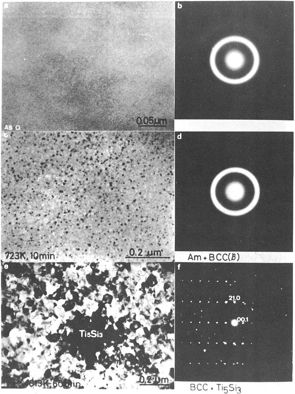
Fig. 28 Transmission electron micrographs and selected area diffraction patterns showing the as-quenched (a and b) and annealed (c, d, e and f) structures of  $Ti_{80}V_5Si_{15}$  amorphous alloy.
