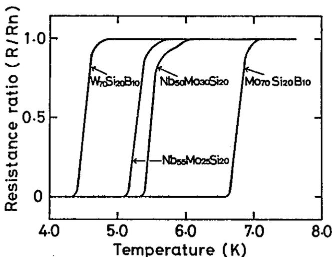
Fig. 10 Resistance ratio  $R/R_n$  as a function of temperature for  $Mo_{70}Si_{20}B_{10}$  and  $W_{70}Si_{20}B_{10}$  amorphous alloys. Also, the data for  $Nb_{55}Mo_{25}Si_{20}$  and  $Nb_{50}Mo_{30}Si_{20}$  amorphous alloys are shown for comparison.
