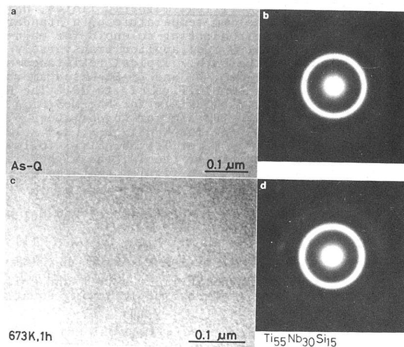
Fig. 16 Transmission electron micrographs and selected area diffraction patterns showing the as-quenched structure (a and b) and the structure after annealing for 1 h at 673 K (c and d) of  $Ti_{55}Nb_{30}Si_{15}$  amorphous alloy.
