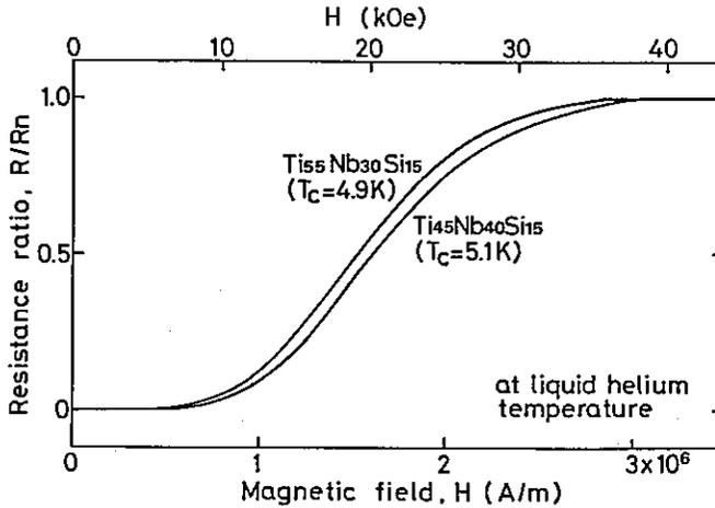
Fig. 19 Resistance ratio  $R/R_n$  as a function of magnetic field at liquid helium temperature for  $Ti_{55}Nb_{30}Si_{15}$  and  $Ti_{45}Nb_{40}Si_{15}$  amorphous alloys.
