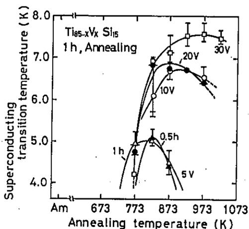
Fig. 31 Changes in superconducting transition temperature ( $T_C$ ) and transition width ( $\Delta T_C$ ) for  $Ti_{85-x}V_xSi_{15}$  amorphous alloys with annealing temperature. Vertical bars represent the transition width.
