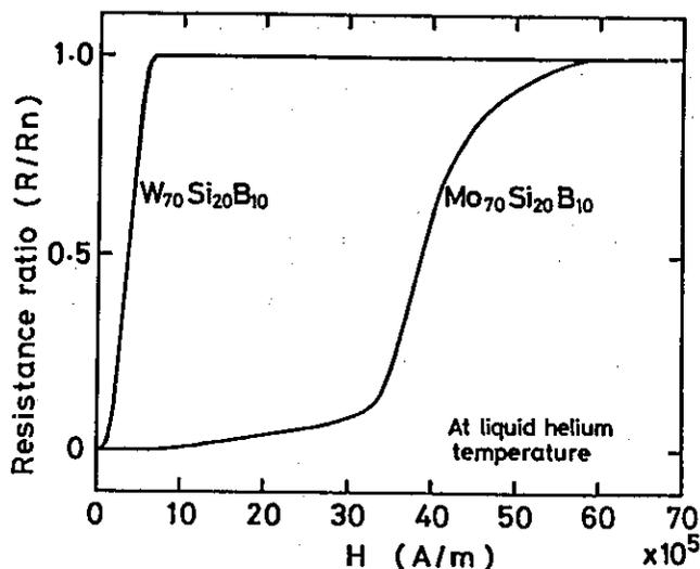
Fig. 18 Resistance ratio  $R/R_n$  as a function of magnetic field at liquid helium temperature for  $\text{Mo}_{70}\text{Si}_{20}\text{B}_{10}$  and  $\text{W}_{70}\text{Si}_{20}\text{B}_{10}$  amorphous alloys.
