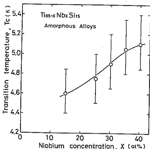
Fig. 11 Niobium concentration dependence of the superconducting transition temperature ( $T_C$ ) and the transition width ( $\Delta T_C$ ) for  $\text{Ti}_{85-x}\text{Nb}_x\text{Si}_{15}$  amorphous alloys. Vertical bars represent the transition width.
