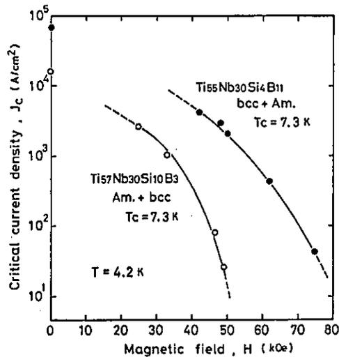
Fig. 21 Critical current density ( $J_c$ ) of  $\text{Ti}_{55}\text{Nb}_{30}\text{Si}_4\text{B}_{11}$  and  $\text{Ti}_{57}\text{Nb}_{30}\text{Si}_{10}\text{B}_3$  amorphous alloys as a function of magnetic field applied normal to the direction of current flow.
