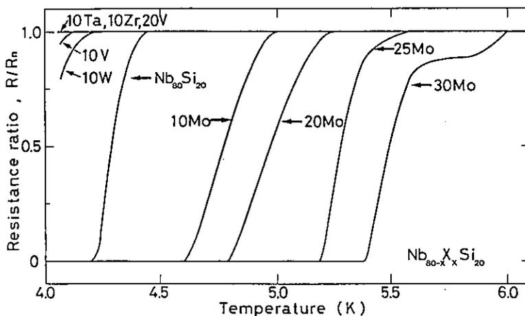
Fig. 9 Resistance ratio  $R/R_n$  as a function of temperature for  $Nb_{80}Si_{20}$  and  $Nb_{80-x}M_xSi_{20}$  ( $M=V, Zr, Mo, Ta$  and  $W$ ) amorphous alloys.
