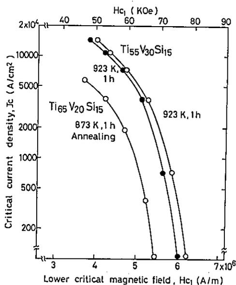
Fig. 36 Critical current density ( $J_c$ ) of  $Ti_{65}V_{20}Si_{15}$  and  $Ti_{55}V_{30}Si_{15}$  amorphous alloys annealed for 1 h at 873 and 923 K as a function of magnetic field applied normal to the direction of current flow.
