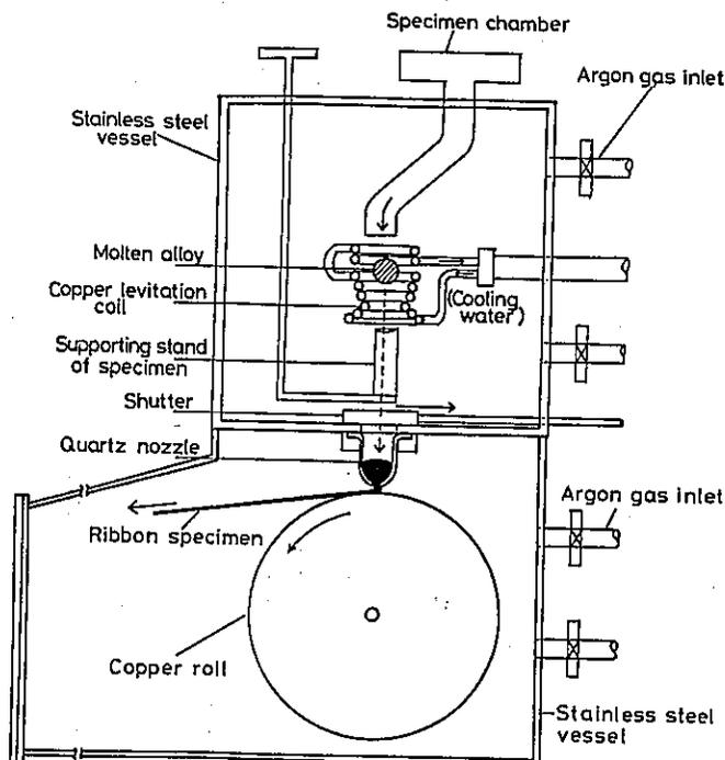
Fig. 1 Schematic illustration of the rapid quenching apparatus used in the present work.
