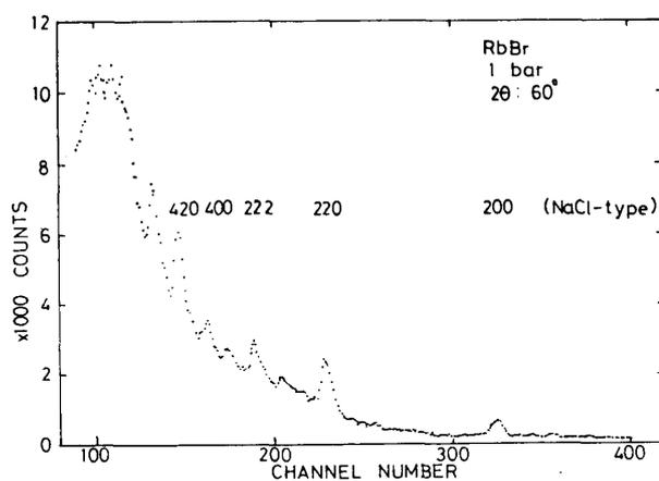
Fig. 7. Neutron diffraction of RbBr powder at 1 bar.
