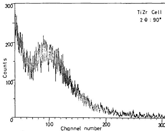
Fig. 4. Spectrum of neutrons scattered by Ti-Zr cell.
