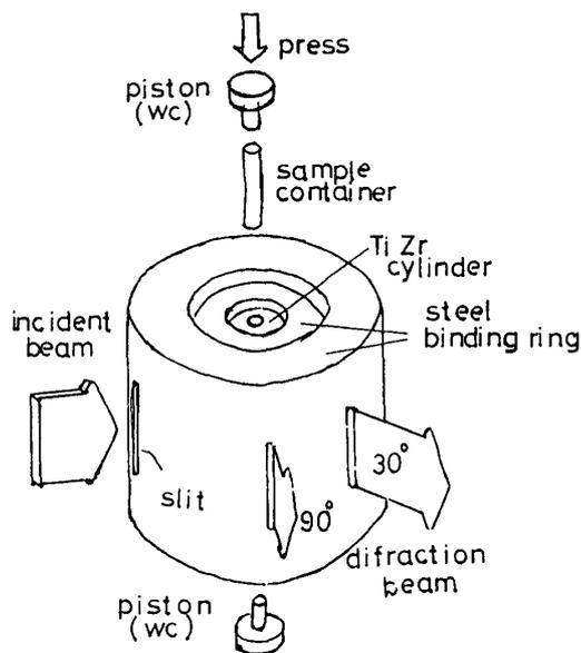
Fig. 2. High pressure apparatus for TOF neutron diffraction.
