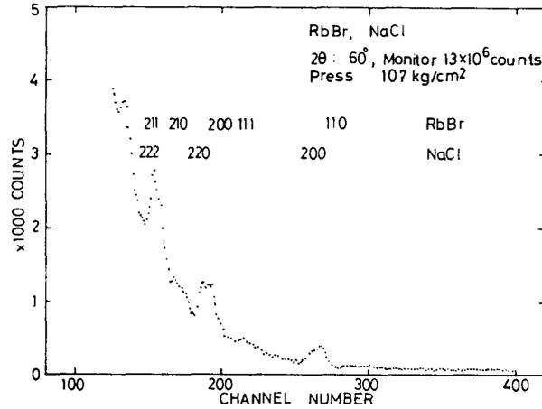
Fig. 9. Neutron diffraction in RbBr and NaCl mixture at high pressure, lines for RbBr are indexed as CsCl-type structure.
