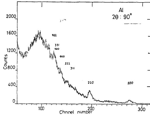
Fig. 5. Scattering of neutrons from polycrystalline aluminum.
