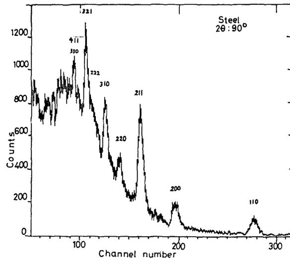
Fig. 6. Scattering of neutrons from polycrystalline iron.
