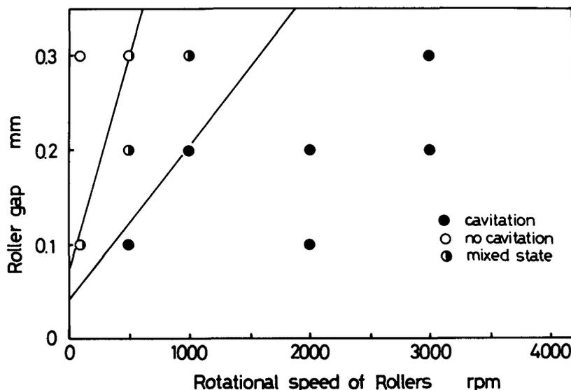
Fig.2 Critical rotational speed of rollers for a cavitation occurrence in liquid as a function of the roller gap in the case of Ni<sub>75</sub>Si<sub>8</sub>B<sub>17</sub> alloy ejected at 1473 K.
