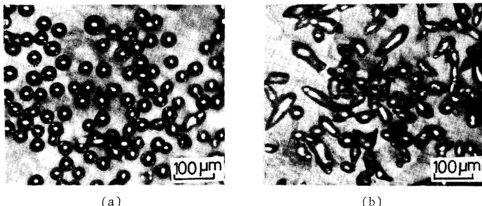
Fig. 4 The shape of  $\text{Ni}_{75}\text{Si}_8\text{B}_{17}$  (a) and  $\text{Fe}_{75}\text{Si}_{10}\text{B}_{15}$  powders (b) sieved under 400 mesh ( $37\ \mu\text{m}$ ). Both samples were produced under the conditions of 5000 rpm of rotational roller speed, 0.1 mm of roller gap and 1773 K of ejecting temperature.
