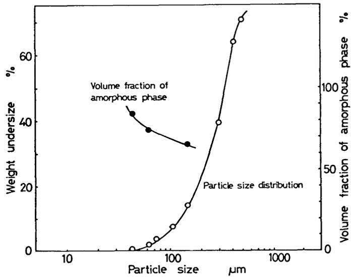
Fig. 6 The relationship between the weight undersize and the particle size for  $\text{Co}_{72.5}\text{Si}_{12.5}\text{B}_{15}$  alloy powders produced at the same conditions described in Fig.5. The volume fraction of amorphous phase is also in the figure.
