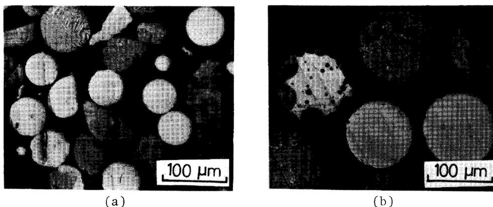
Fig. 7 Microstructures of Ni<sub>75</sub>Si<sub>8</sub>B<sub>17</sub> alloy powders with the size of 44-63 μm (a) and 105-149 μm (b), produced at the conditions of 5000 rpm, 0.1 gap and 1623 K of ejecting temperature.
