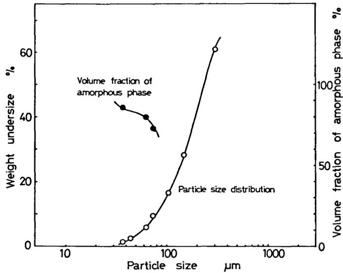
Fig. 5 The relationship between the weight undersize and the particle size for  $\text{Ni}_{75}\text{Si}_8\text{B}_{17}$  alloy powders produced at the roller speed of 5000 rpm, the roller gap of 0.1 mm and the ejecting temperature of 1773 K. The volume fraction of amorphous phase is also shown in the figure.
