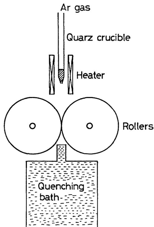
Fig. 1 Schematic diagram of a twin-roller type apparatus used.
