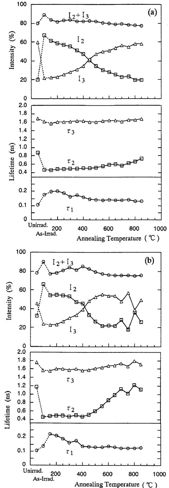
Fig. 5 Annealing behavior of the positron lifetime parameters for (a) HRP, and (b) ES.
