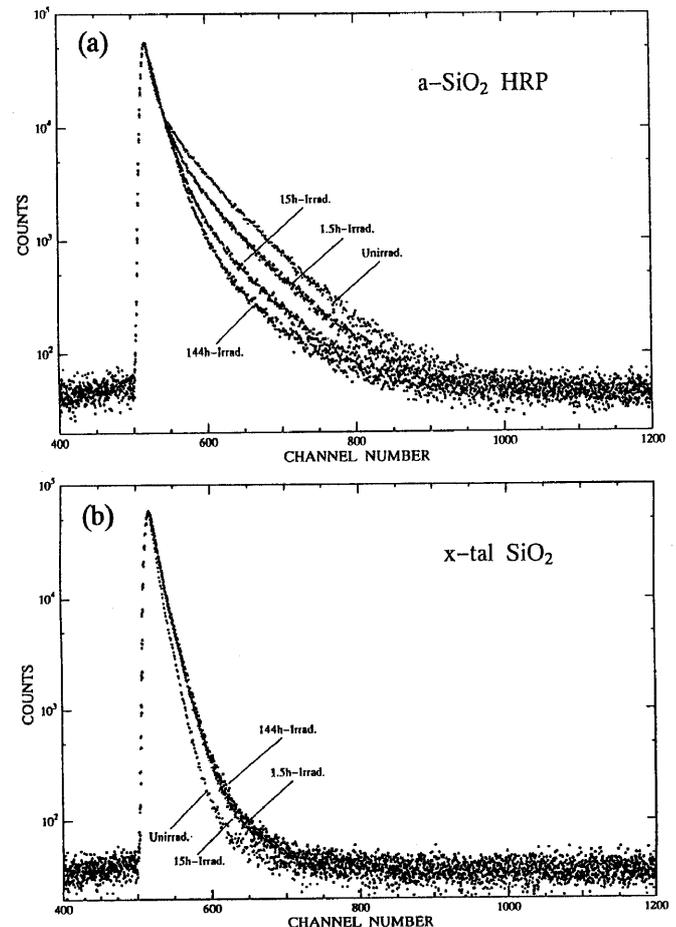
Fig. 1. Positron lifetime spectra for (a) the HRP silica glass, and (b) quartz single crystals. Fast-neutron doses are  $8.6 \times 10^{16}$  n/cm<sup>2</sup> (1.5h),  $8.6 \times 10^{17}$  n/cm<sup>2</sup> (15h), and  $8.3 \times 10^{18}$  n/cm<sup>2</sup>. The time scale is 25.62 ps/channel.
