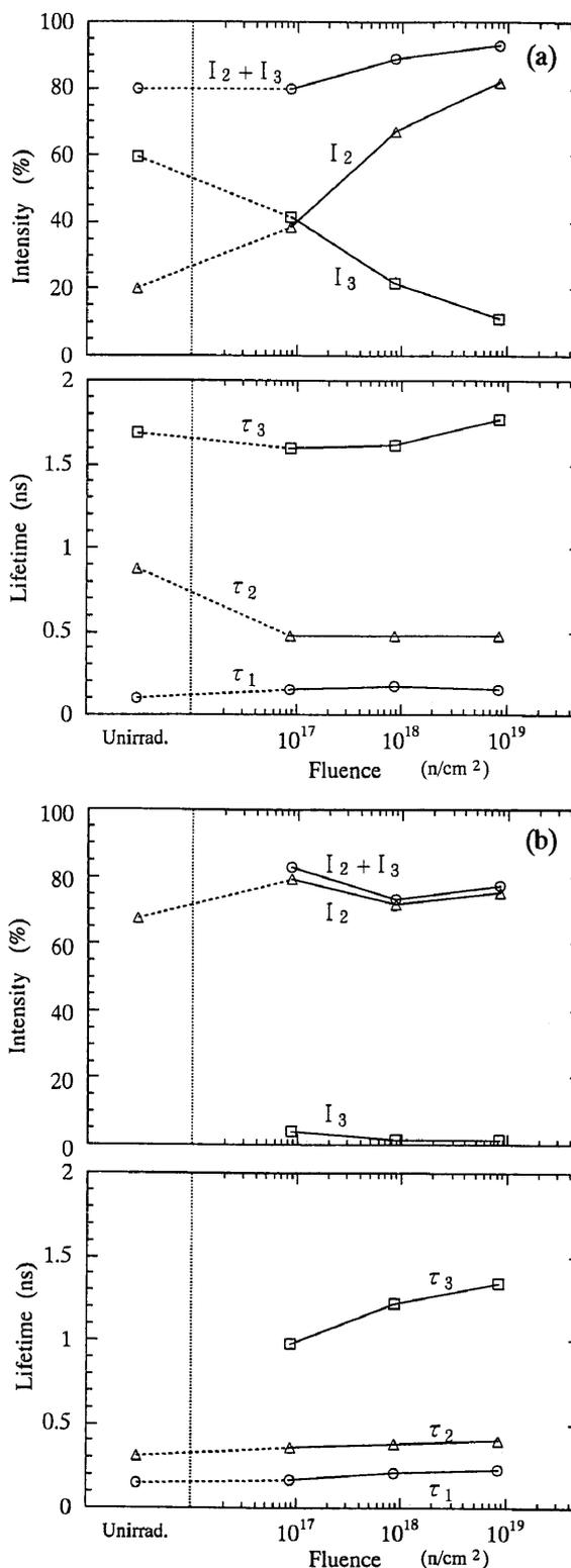
Fig. 2. Fast-neutron dose dependence of positron lifetimes and their relative intensities for (a) the HRP silica glass, and (b) quartz single crystal.
