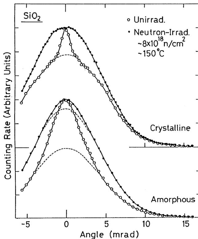
Fig. 4 ACAR curves for quartz crystals and silica glass before and after neutron-irradiation of  $8.3 \times 10^{18} \text{ n/cm}^3$ . For silica glass dashed lines show the deconvolution into two Gaussian components by a least-square fitting.
