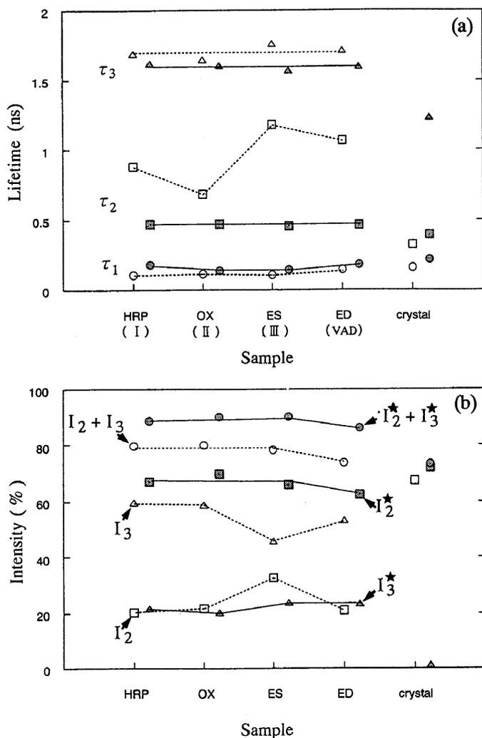
Fig. 3 Variation of the positron lifetime parameters in samples used. Open circles, squares and triangles stand for unirradiated samples, and dotted symbols for neutron-irradiated ones with a dose of  $8.3 \times 10^{17} \text{ n/cm}^2$ . The intensities  $I_i$  for the irradiated samples are asterisked. Results for the crystal are also displayed.
