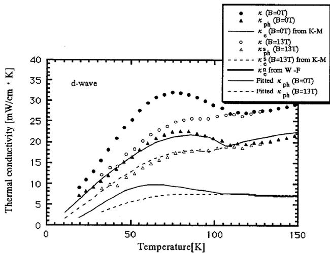
Figure.5 Comparison of the temperature dependence of the thermal conductivity with the calculated one on the basis of the coexisting model.
