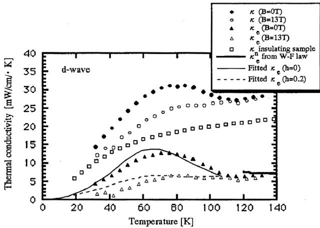
Figure.3 Comparison of the temperature dependence of the thermal conductivity with the fitted curve using the modified K-M expression.
