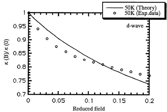
Figure.6 Comparison of the field dependence of the thermal conductivity with the calculated one on the basis of the coexisting model.
