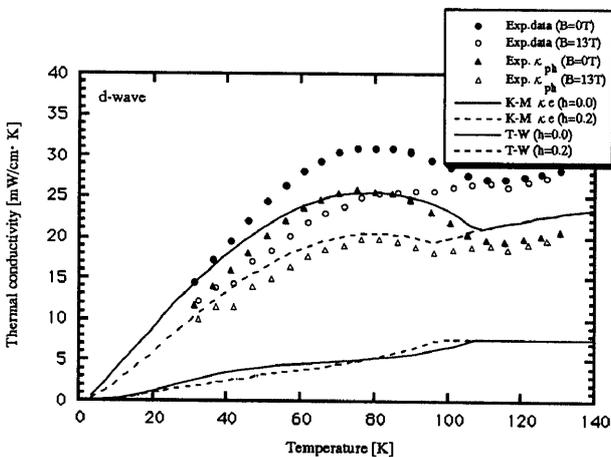
Figure.1 Comparison of the temperature dependence of the thermal conductivity with the calculated one on the basis of the conventional superconductor model.
