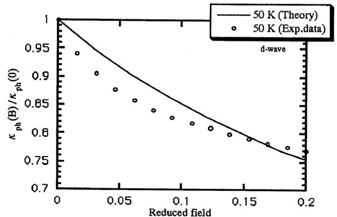
Figure.2 Comparison of the field dependence of the thermal conductivity with the calculated one on the basis of the conventional superconductor model.
