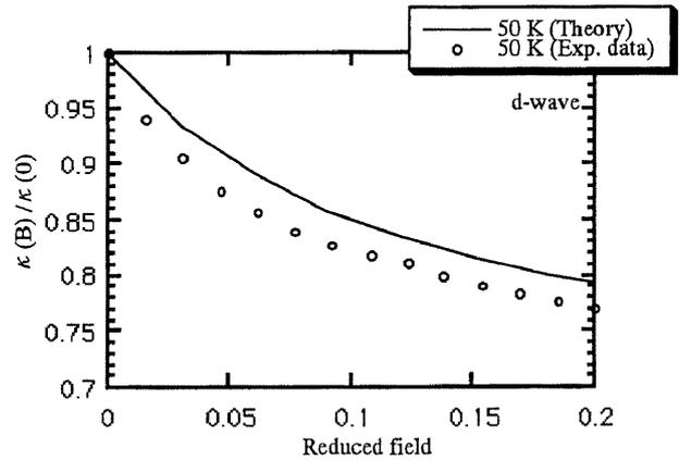
Figure.4 Comparison of the field dependence of the thermal conductivity with the calculated one on the basis of the modified K-M expression.
