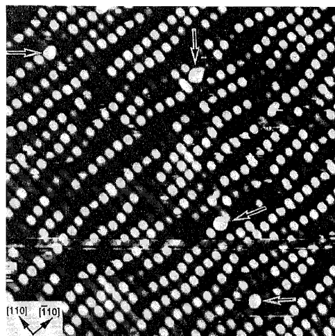
Figure 29. The close-up filled states STM image ( 490\text{\AA} \times 490\text{\AA} ) of the newly defined 4 \times 1 phase. The arrows indicates four larger Ga clusters (Ga droplet precursors) compared with the regular size ones.
