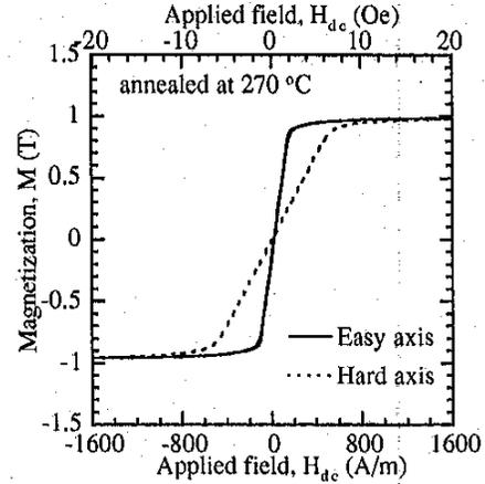
Fig. 3. Magnetization curve of the CoNbZr film.
