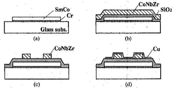
Fig. 4. Fabrication steps of the integrated sensor: (a) sputter and ion milled SmCo/Cr layer; (b) sputter CoNbZr/SiO<sub>2</sub> layer; (c) ion mill CoNbZr layer; (d) sputter Cu legs.
