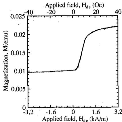
Fig. 5. Magnetization curve of CoNbZr/SmCo bilayer film.
