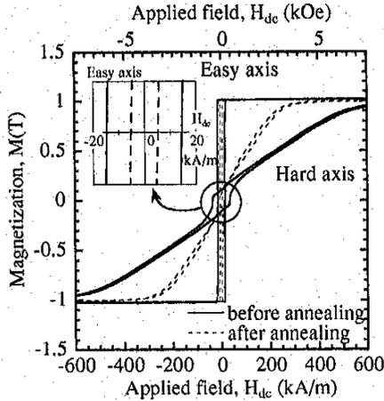
Fig. 2. Magnetization curve of the SmCo film.
