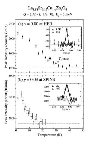
FIG. 3. Temperature dependence of the incommensurate elastic magnetic peak intensity at  $Q=(\frac{1}{2}-\epsilon,\frac{1}{2},0)$  for (a) y=0.00 (filled circles) and (b) y=0.03 (open circles) crystals. Note that two different spectrometers, that is, HER and SPINS were used for the y=0.00 and y=0.03 samples, respectively. The inset in each figure shows peak profiles around  $(\frac{1}{2}-\epsilon,\frac{1}{2},2)$  at high and low temperatures.
