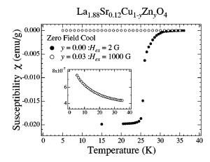
FIG. 1. Magnetic susceptibility measured after cooling in zero field for single crystals with y = 0.00 (filled circles) and y = 0.03 (open circles). The inset shows the detailed temperature dependence of the susceptibility for the y = 0.03 crystal.
