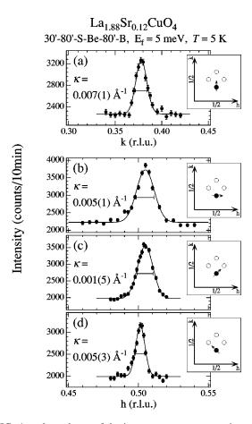
FIG. 4. q dependence of the incommensurate magnetic peak in the crystal with y=0.00 which was measured through the peak at  $Q=(\frac{1}{2},\frac{1}{2}-\epsilon,0)$  at T=5 K. The arrow in the inset of each figure shows the direction of each scan. The solid line in each figure shows the result of fitting a Gaussian profile convoluted with the instrumental resolution as discussed in the text. The solid short line in each figure shows the width of the resolution at the peak position.
