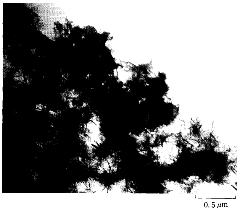
Photo. 3 Transmission electron microscopic observation of metallic Fe ultrafine particles synthesized from \text{Fe}(\text{CH}_3\text{COCHCOCH}_3)_3 with \text{LiAlH}_4 in tetrahydrofuran.
