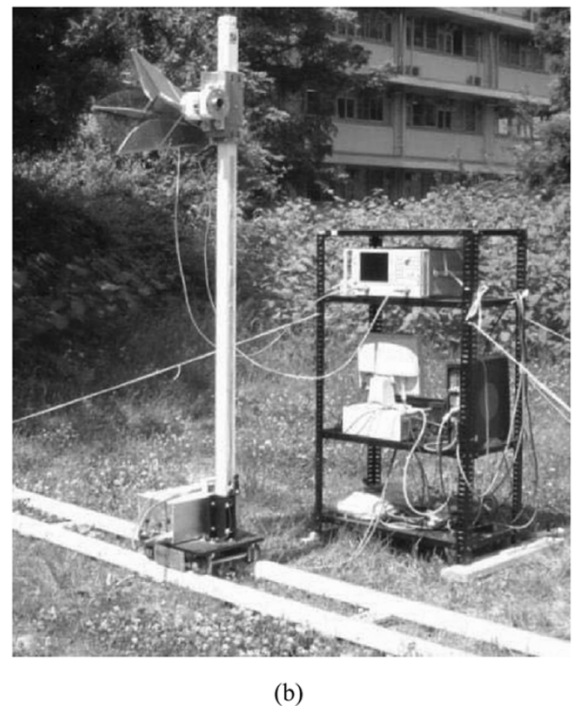
Fig. 1. Configuration of the broadband ground-based polarimetric SAR system. (a) A schematic and (b) photograph of the developed system as built.
