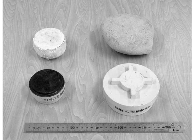
Fig. 7. GPR targets. Plastic foam, stone, PMN-2, and Type 72.
