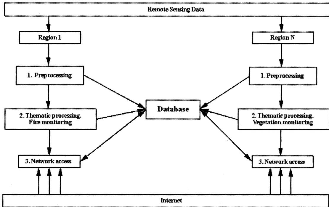
Fig. 10 General scheme of distributed satellite data storing and processing system
