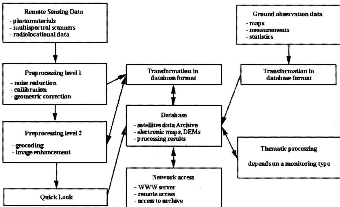
Fig. 11. The scheme of distributed satellite data storing and processing system
