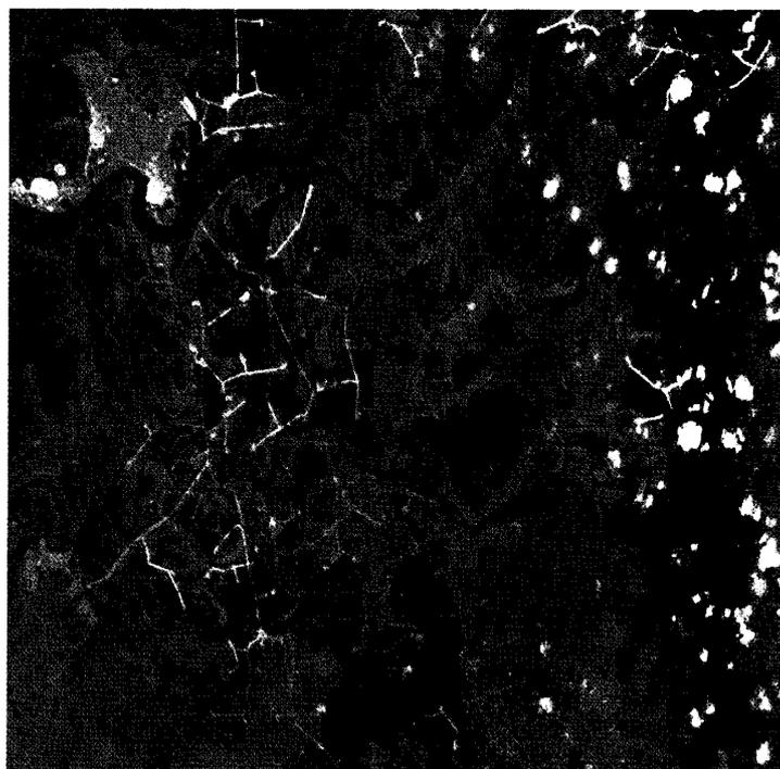
Fig. 3. Example of saturation by pipelines and technogenic objects for an oil deposit in West Siberia. Resurs O1 N3 satellite image. Resolution 40 meters. Size of region is 40x40 km.
