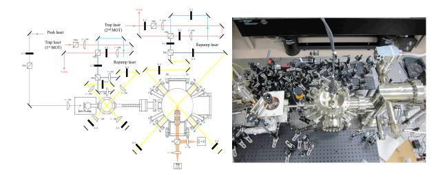
Figure 1. The experimental setup of the double MOT. The left figure shows the configuration of the MOT chambers and laser. The right picture shows the developed experimental apparatus of the double MOT.
