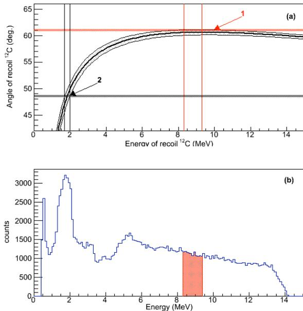
Figure 1. (a) The kinematic calculation of the recoil  $^{12}\text{C}$  energy and angle. (b) The energy spectrum obtained in the SSD0 detector. The red-hatched region corresponds to the excitation energy of about 16.5 MeV in  $^{16}\text{O}$ .
