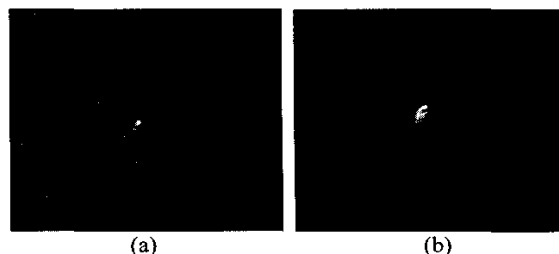
Fig. 7. Electron emission pattern at the tip-anode distance of 2 mm (spot size ~ 1 mm) (a) and 35 mm (b).
