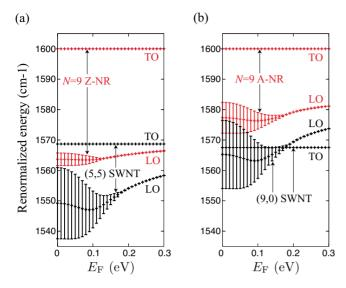
FIG. 3. (Color online) (a) The  $E_{\rm F}$  dependence of the renormalized energies of the LO and TO modes in a N=9 Z-NR and of the LO and TO modes in a (5,5) SWNT. (b) The  $E_{\rm F}$  dependence of the renormalized frequencies of the LO and TO modes in a N=9 A-NRand of the LO and TO modes in a (9,0) SWNT.
