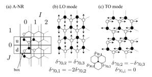
FIG. 4. (a) The lattice structure of an A-NR. (b) and (c) The eigenvectors of the  $\Gamma$  point LO and TO phonon modes are illustrated. The LO mode satisfies  $\delta\gamma_{0,1}=-2\delta\gamma_{0,2}$  and  $\delta\gamma_{0,2}=\delta\gamma_{0,3}$ . The TO mode is characterized by  $\delta\gamma_{0,1}=0$  and  $\delta\gamma_{0,2}=-\delta\gamma_{0,3}$ .
