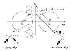
FIG. 6. In the k space, we consider a state near the K point (solid circle) and states, which are scattered by the zigzag and armchair edges (empty circles).  $k_x$  ( $k_y$ ) is taken as parallel to the zigzag (armchair) edge. The arrows in the insets indicate the direction of the pseudospins. The  $\langle \sigma_y \rangle$  component of the pseudospin is reversed at the zigzag edge, while the  $\langle \sigma_x \rangle$  component is preserved at the armchair edge.
