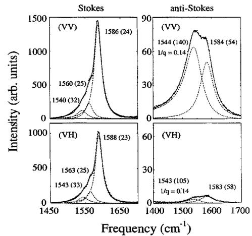
FIG. 2. SERRS spectra from a nonoriented SWNT sample ( $d_t = 1.49 \pm 0.20$  nm) using  $E_l = 830$  nm (1.49 eV) laser excitation. The frequencies (widths) of the Raman peaks are displayed in  $\text{cm}^{-1}$ .
