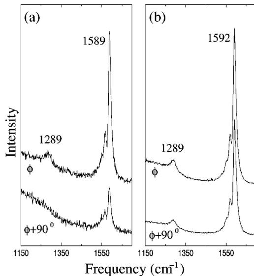
FIG. 4. (a) SERRS spectra from an “invisible” bundle of aligned semiconducting SWNT’s, for two  $VV$  polarization directions separated by  $90^\circ$ , where  $\phi$  denotes a relative maximum of the scattering power. (b) Similar RRS measurements performed on a sample containing many unaligned SWNTs. The frequencies for the  $D$  band and the most intense  $G$  band Raman peak are displayed in  $\text{cm}^{-1}$ .
