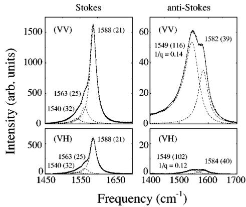
FIG. 1. RRS spectra from a nonoriented SWNT sample ( $d_t = 1.49 \pm 0.20$  nm) using  $E_l = 830$  nm (1.49 eV) laser excitation. The frequencies (widths) of the Raman peaks are displayed in  $\text{cm}^{-1}$ .
