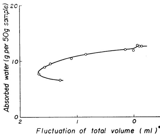
Fig. 4. The relation between the values which were measured by the total volume method and the values measured by the weighing method in the case of **Sasasigure**.
