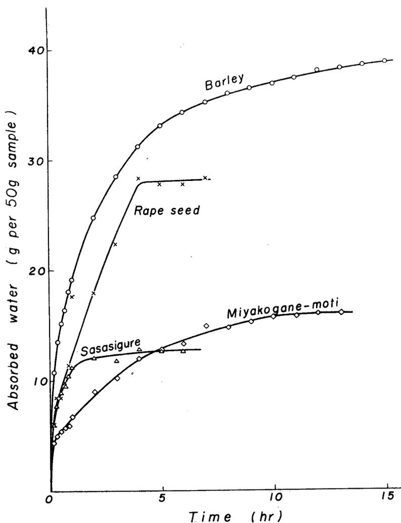
**Fig. 2.** The swelling velocities of barley, two kinds of rice and rape seed by the weighing method.
