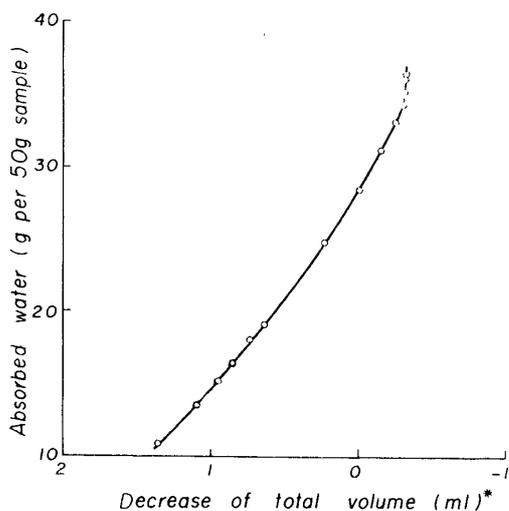
Fig. 3. The relation between the values which were measured by the total volume method and the values measured by the weighing method in the case of **barley**.
