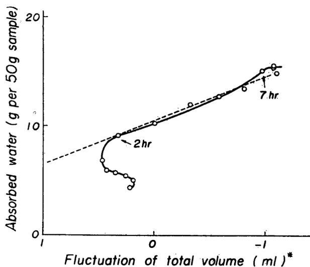
Fig. 5. The relation between the values which were measured by the total volume method and the values measured by the weighing method in the case of **Miyakogane-moti**.
