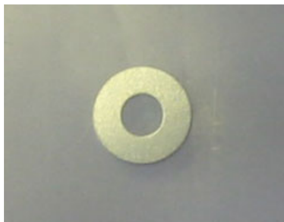
Figure 3.10 Picture of a shim that was used for adjustment of the focus. Shim such as shown in this figure was inserted between the optical units and CCD board (see Figure 2.8 and Figure 3.8).
