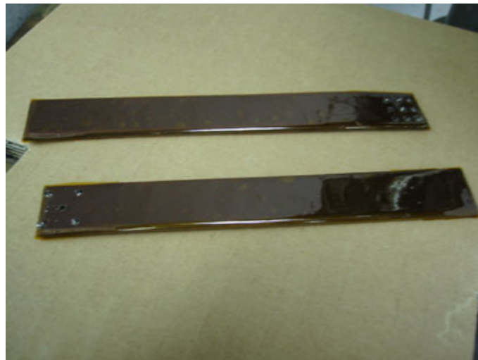
Figure 3.1 Picture of bundles of 20 stacked graphite sheets used as a thermal path for cooling of CCD. It is covered with kapton tape. One side of the graphite sheets bundle is attached to the backside of CCD with an oxygen-free copper block, and the other end is attached to the radiation plate (Figure 3.3), which is placed facing to the space right behind the satellite panel, with aluminum block (Figure 3.2).
