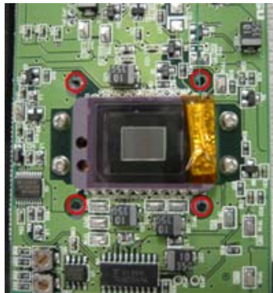
Figure 3.8 A picture of CCD board of MAC. Four red circles denote the point of screw cramp that connects each CCD board to the optical unit.
