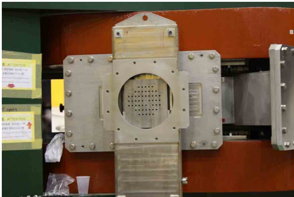
Figure 3.25: Picture of HKS Sieve Slit mounted on the exit of kaon side.
