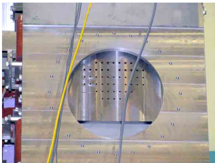
Figure 3.48: Picture of HES Sieve Slit mounted on the entrance of EQ1.
