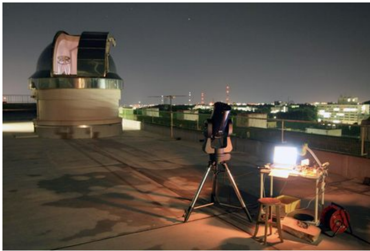
Figure 4.13: Simultaneous observations with Tohoku DIMM (inside the astronomical dome) and the Hiroshima University Differential Image Motion Monitor (HU-DIMM) at right side.
