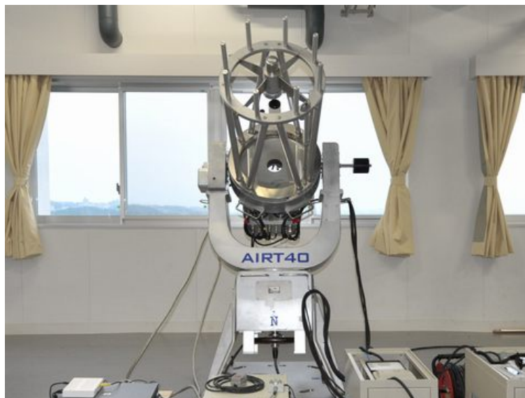
Figure 4.8: Antarctic Infra-Red Telescope with a 40 cm primary mirror (AIRT40) under assembling in the laboratory at the end of August 2010.
