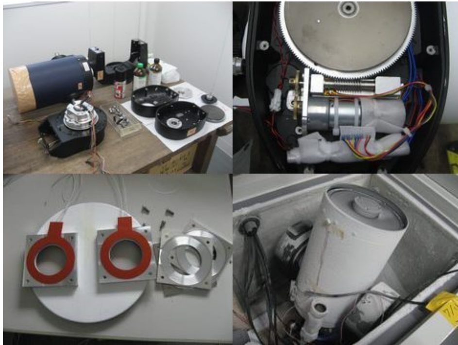
Figure 4.19: Left top; Complete disassembling of LX200 for modifying the cold environment. Right top; Motor and electric circuit with heater and polyurethane form (white, wrapping one). Left bottom; “Doughnut-shape” heaters for optical windows. Right bottom; Cold test for LX200 in a freezer.
