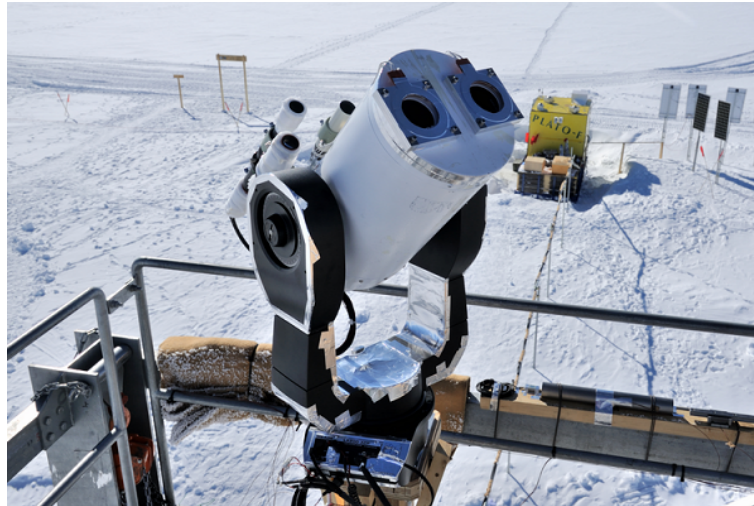
Figure 4.18: DF-DIMM on the 9-m astronomical tower at Dome Fuji, 2013 January. Copyright: Okita et al. (2013a) [50]
