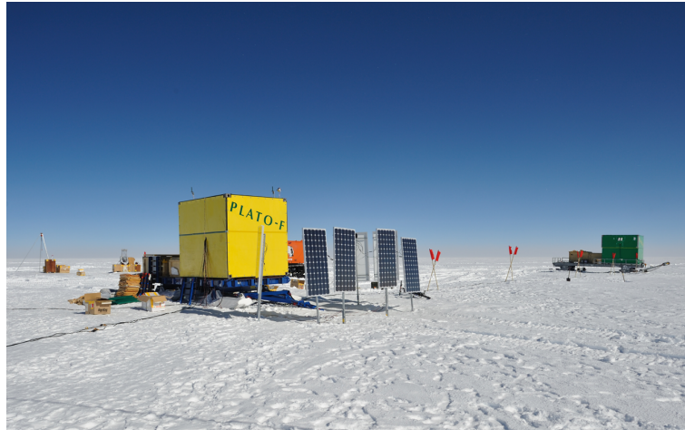
Figure 4.2: PLATO-F at Dome Fuji in January 2011. The left yellow and right green containers are the Instrument Module and Engine Module, respectively. The solar panels are seen in front of the Instrument Module.
