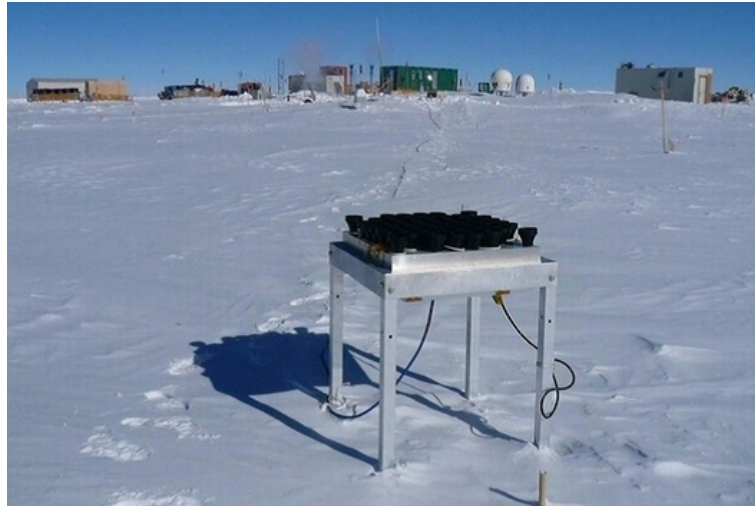
Figure 4.1: Remtech Inc. #PA-1 SODAR without sound cone set at Dome Fuji station in 2006. The backgrounds behind #PA-1 SODAR are the buildings of the station.
