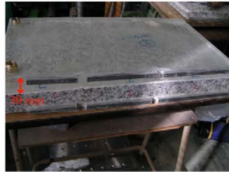
(g) Final desire height and matching tool is glued
