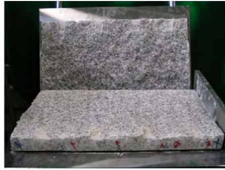
(b) Creating a tensile fracture in a block of size 530 mm x 300 mm x 200 mm
