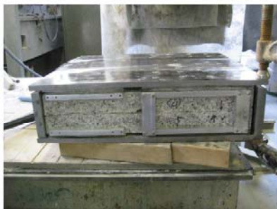
(c) Assembling of reference plate with the sample
