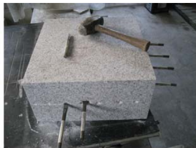
(a) Creating a tensile fracture in a block of size 385 mm x 385 mm x 200 mm
