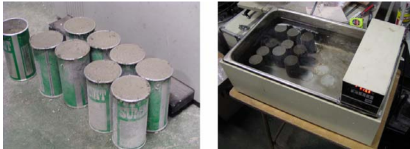
Fig. 5.1. Making and preparing the mortar core samples to be tested.
