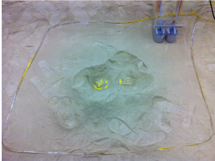
Fig. 5.8. GPR experiment configuration using two landmines as targets.
