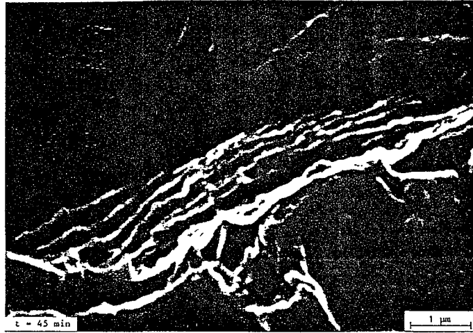
Fig. 4 Fracture surface showing a fatigue striations
