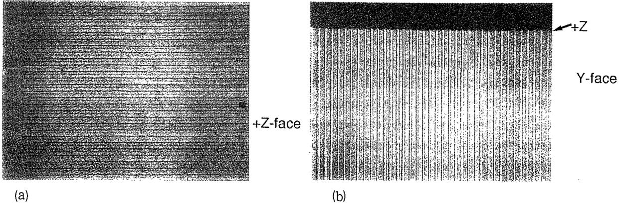
Fig. 2 Photograph of the etched faces of the periodically domain inverted Nd:LT laser. (a) show the +z face (b) the y face, the wider strips are those under the electrodes and experience domain reversal. Thickness is 500 μm and period is 8.1 μm.
