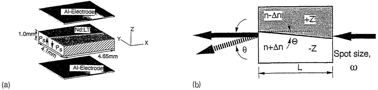
Fig. 1 Geometry of the integrated electro-optic Q-switching and lasing crystal. The axis of optical propagation is x, and the electric field is applied along z. The angle of inclination  $\Theta$  of the boundary is  $3^\circ$ . (a) Exploded view. (b) Schematic explaining the deflection caused by the domain boundary under the applied field.
