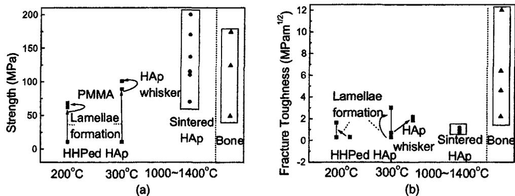
Fig.3 Strength (a) and fracture toughness (b) of the hydroxyapatite ceramics
