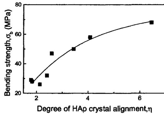
Fig.2 Relationship between bending strength and degree of HAp crystal alignment
