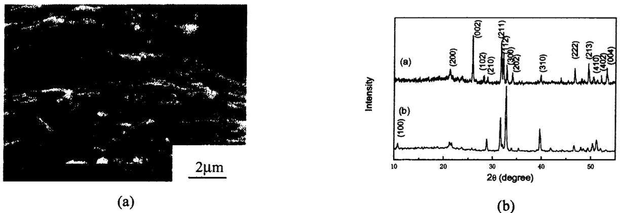
Fig.1 SEM photograph (a) and XRD pattern (b) of the sample fabricated from OCP and ammonia water
