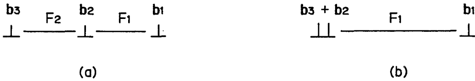
Fig. 1. Possible core extension of a 1/3\langle\bar{1}1\bar{2}3\rangle dislocation on \{10\bar{1}1\} . (a) Dissociation into three partial dislocations b_3 , b_2 and b_1 with the two enclosed stacking faults F_2 and F_1 . (b) Dissociation into two partial dislocations (b_3+b_2) and b_1 with the fault F_1 .
