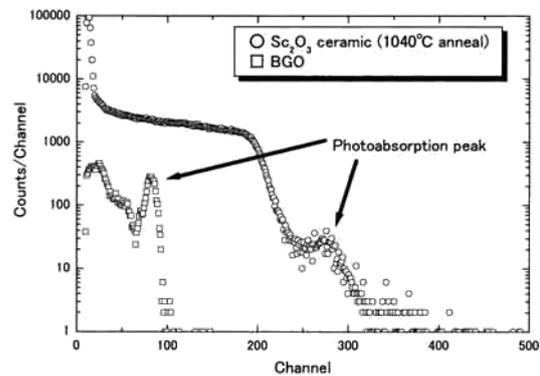
Fig.4. Pulse height spectra of  $\text{Sc}_2\text{O}_3$  ceramic under  $^{137}\text{Cs}$  excitation together with BGO data as a reference.
