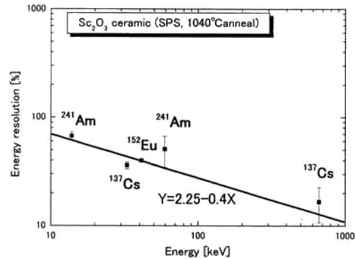
Fig.6. Energy resolution of  $\text{Sc}_2\text{O}_3$  ceramic using various  $\gamma$ -ray emitters
