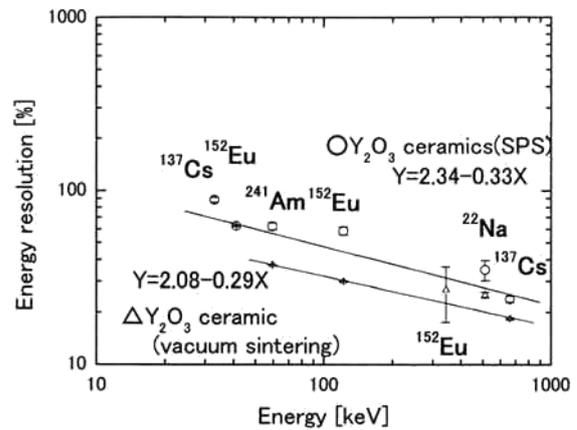
Fig.3. Energy resolution plots of  $\text{Y}_2\text{O}_3$  ceramics using various  $\gamma$ -rays emitters.
