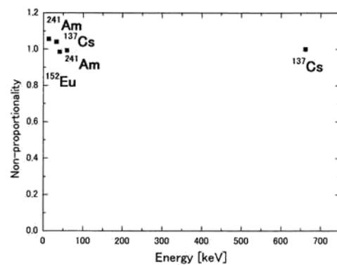
Fig.5. Non-proportionality plots of  $\text{Sc}_2\text{O}_3$  ceramic using various  $\gamma$ -rays emitters.
