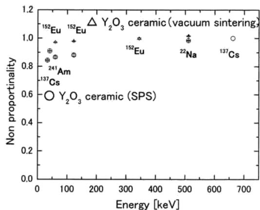
Fig.2. Non-proportionality plots of  $Y_2O_3$  using various  $\gamma$ -rays emitters.
