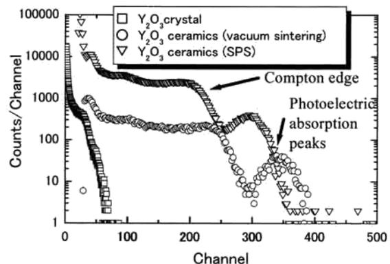
Fig. 1. Pulse height spectra of  $Y_2O_3$  under  $^{137}Cs$  excitation.
