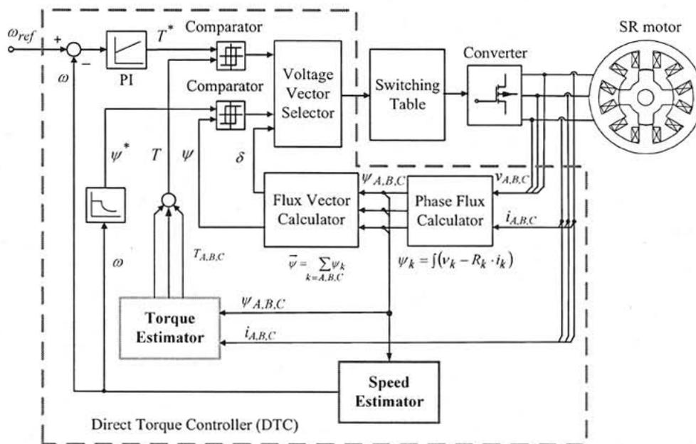
Fig. 2. Proposed position sensorless DTC for SR motors
