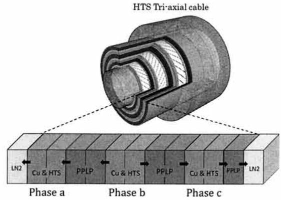
Fig. 5 Unsymmetrical cooling configuration of tri-axial cable.
