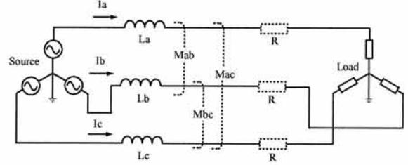
Fig. 2 Equivalent circuit.
