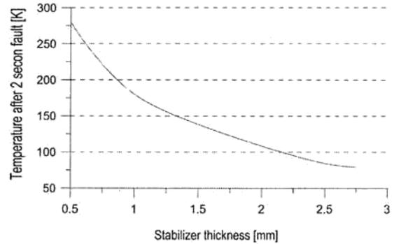
Fig. 6 Cable max temperature as a function of copper stabilizer thickness.
