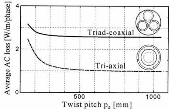
Fig. 4 AC loss comparison between 1layer/phase tri-axial and triad-coaxial cable.
