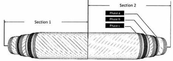
Fig. 1 Two-section tri-axial HTS cable.
