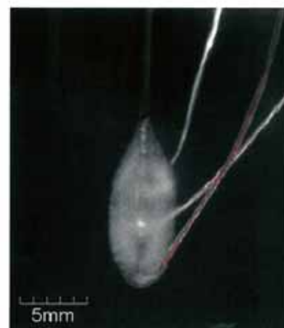
Fig. 3 Snapshot of frozen region around ultrafine cryoprobe in 180 seconds
