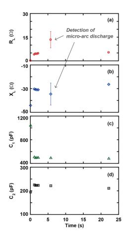
Fig. 4 Time variations of (a) real part of load impedance  $R_L$ , (b) imaginary part of load impedance  $X_L$ , (c) capacitance of variable capacitor  $C_I$ , (d) capacitance of variable capacitor  $C_2$ .
