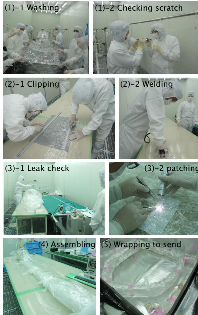
Figure 4.4.: Pictures of the IB fabrication process. (1)-1 Washing a film by ultrasonic cleaning with pure water. (1)-2 Checking scratches and pin holes. (2)-1 Clipping films a gore. (2)-2 Welding films. (3)-1 Checking leakage from the IB with He detector. (3)-2 Patching in a leak spot. (4) Assembling the IB, connection pipe, supporting film belts and Vectran strings. (5) Wrapping the IB and packing into the plastic box. ( A. Gando, 2012 [40] ).
